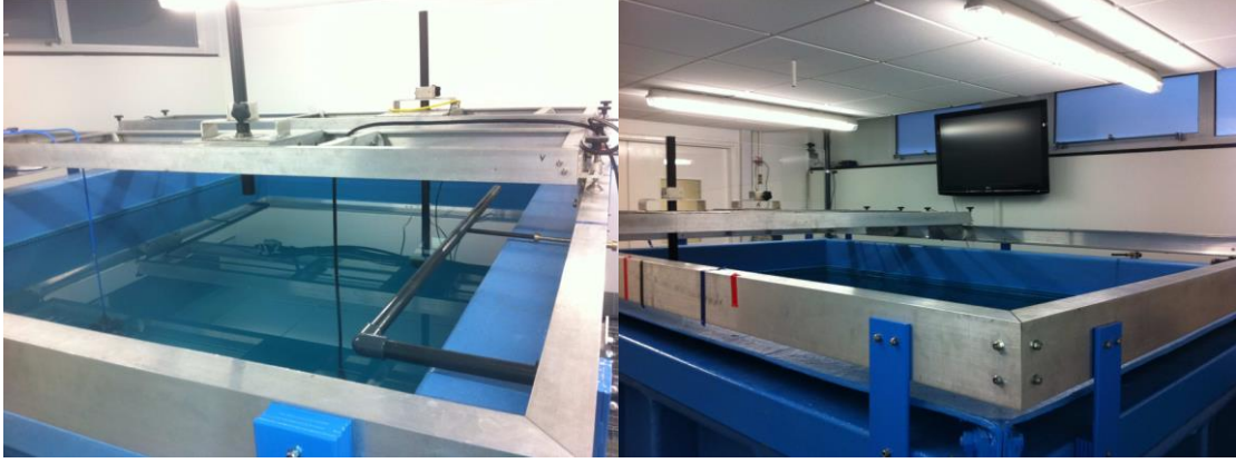
Figure 4.7: Newcastle University Sensors Electromagnetics and Acoustics Laboratory (SEA Lab) Anechoic Testing Tank.
