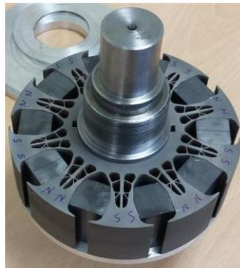
Figure 8-17 Simplified single piece rotor prototype.
