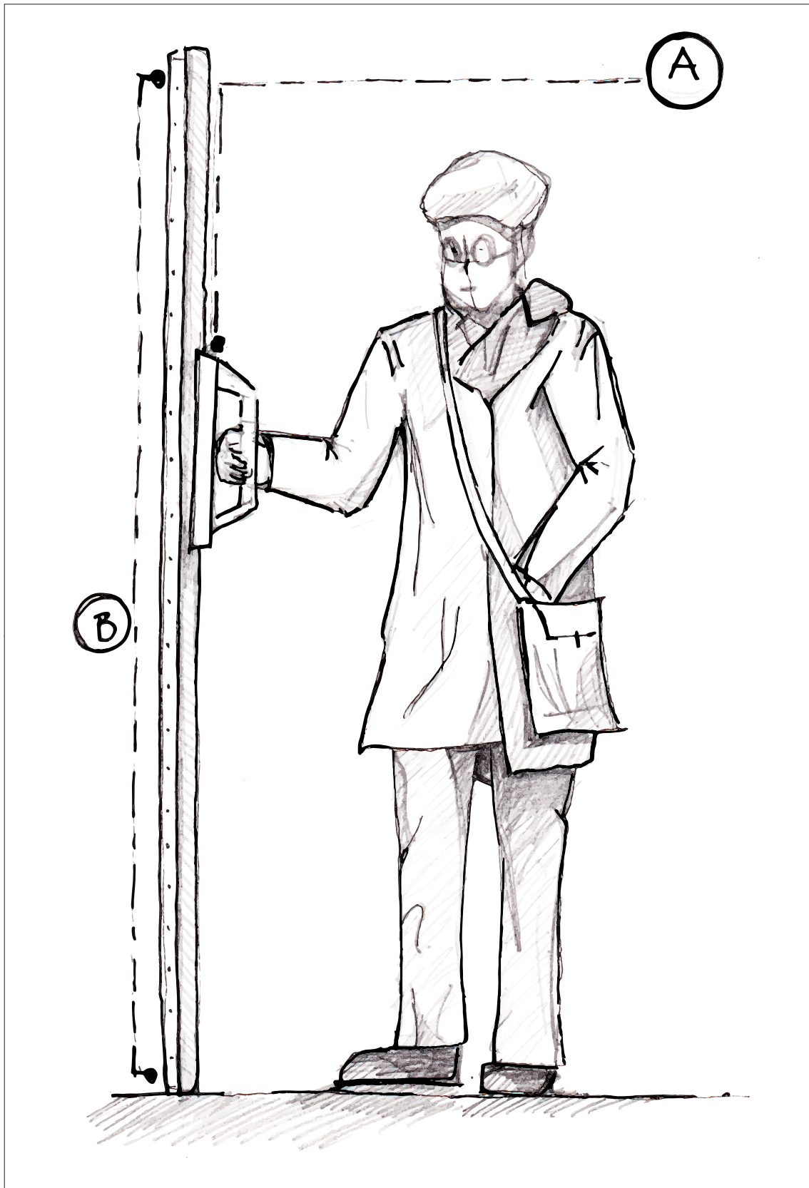
4 Diagram showing the sensor at a fixed height (labelled A), and how it is mapped to a stack of LEDs (labelled B)
