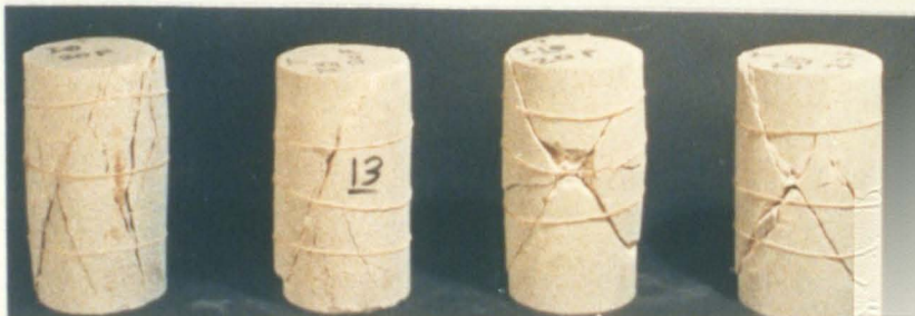
Plate 7.3 Fractured and deformed unjointed SS specimens, strain rate= 8.33 \times 10^{-4} , confining pressure, left to right, 0, 5, 10 & 15 MPa.
