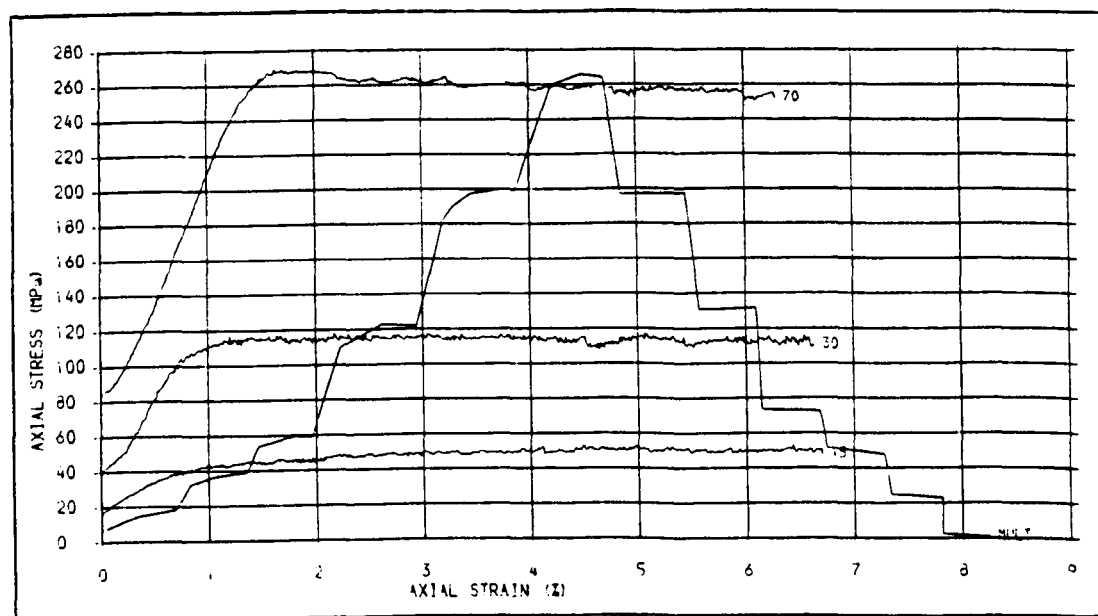
Fig. 678 .STRESS-STRAIN PLOTS FOR PS SPECIMENS WITH SAW CUT JOINTS, JOINT ANGLE= 60 DEG. ONE AND MULTI-STAGE TESTS, CONFINING PRESSURES. 5, 10, 15, 30, 50 AND 70 MPa.
