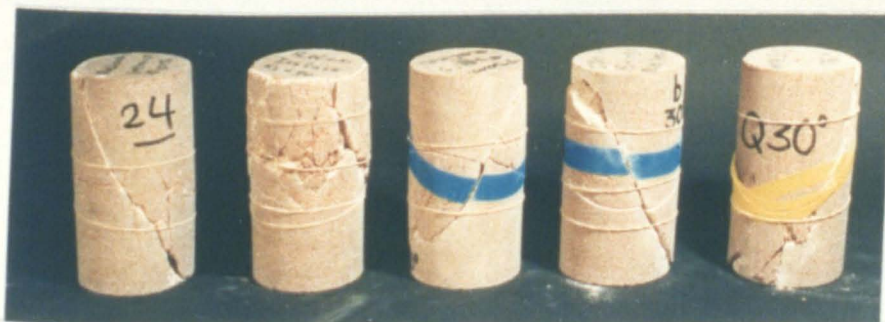
Plate 7.11 Fractured and deformed PS specimens under different loading conditions, joint angle and type of joint, left to right: intact (1 & 2); 30^\circ , saw cut (3 & 4); 30^\circ , natural (5), type of loading: relaxation, confining pressure: 15, 30, 15, 30 & 30 MPa.
