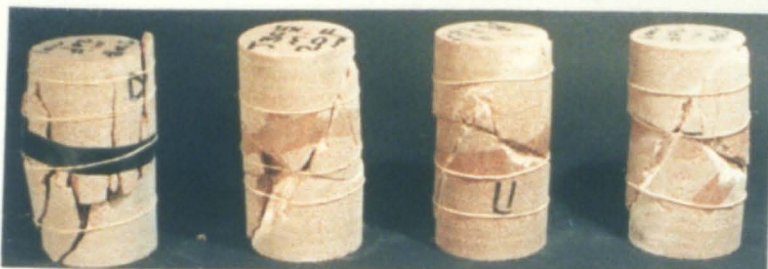
Plate 7.9 Fractured and deformed PS specimens, joint angle= 30^\circ , strain rate= 8.33 \times 10^{-5} , confining pressure, left to right, 0, 5, 10 & 15 MPa.
