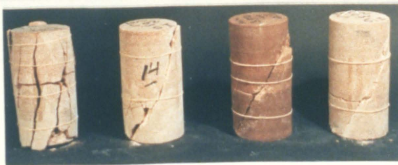
Plate 7.8 Fractured and deformed unjointed PS specimens, strain rate = 2.08 \times 10^{-6} , confining pressure, left to right, 0, 5, 10 & 15 MPa.
