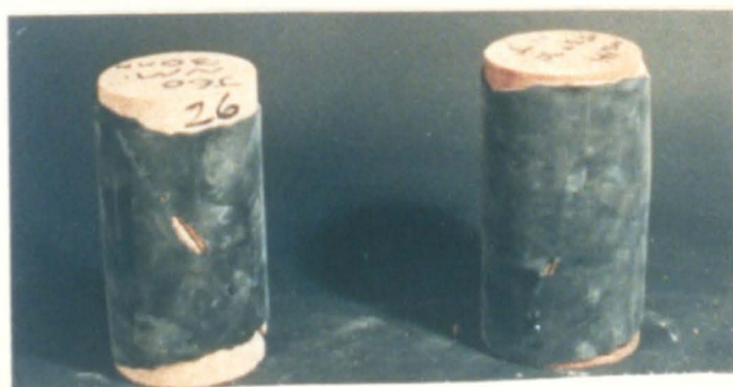
Plate 3.5 Rupture of single membrane during the deformation of specimen or sliding along joint plane.
