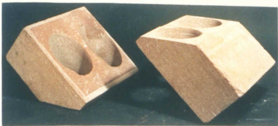
Plate 3.3 Blocks of rock after coring of natural joint.
