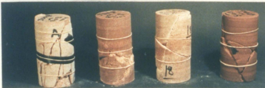
Plate 7.7 Fractured and deformed unjointed PS specimens, strain rate = 2.08 \times 10^{-6} , confining pressure, left to right, 0, 5, 10 & 15 MPa. Joint angle = 30^\circ
