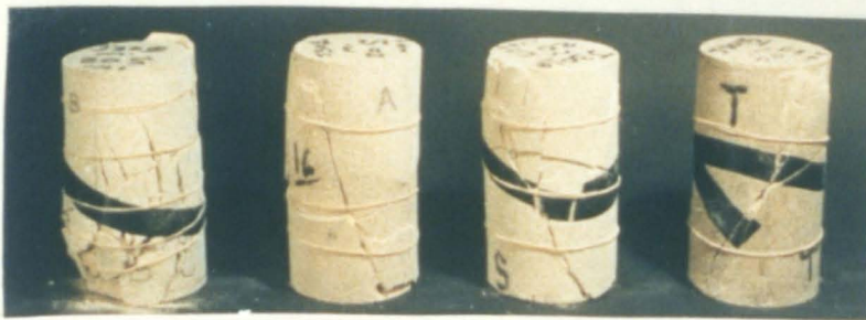
Plate 7.5 Fractured and deformed SS specimens, joint angle = 30^\circ , strain rate = 2.08 \times 10^{-6} , confining pressure, left to right, 0, 5, 10 & 15 MPa.
