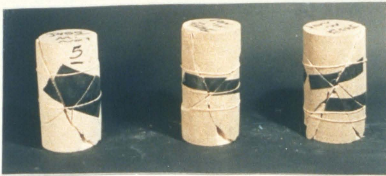
Plate 6.4 Fractured and deformed SS specimens with saw cut joint, confining pressure, left to right, 5, 10, & 15 MPa, joint angle = 45^\circ .
