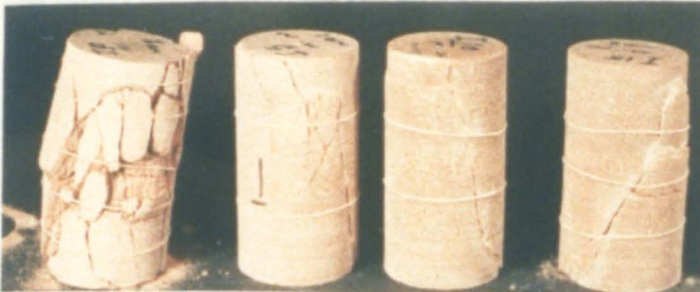
Plate 7.6 Fractured and deformed unjointed PS specimens, strain rate = 4.16 \times 10^{-6} , confining pressure, left to right, 0, 5, 10 & 15 MPa.
