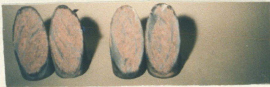
Plate 9.3 Sliding surfaces of slate specimens with saw cut joints, confining pressure, left to right, 70 & 30 MPa.
