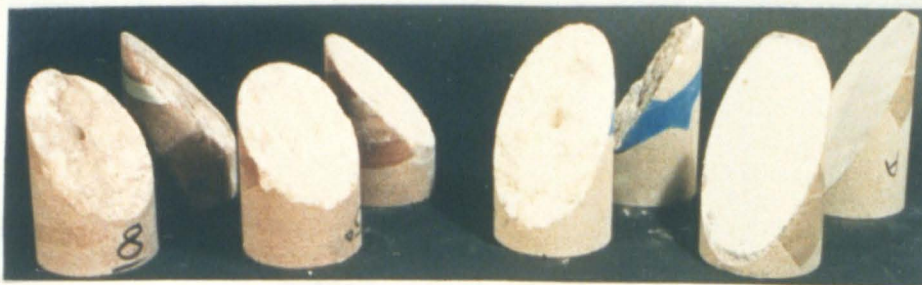
Plate 6.7 Natural and artificial joint sections after sliding and deforming along joint plane, joint angle = 45° & 60°, confining pressure, left to right, 30, 15, 30 & 15 MPa.
