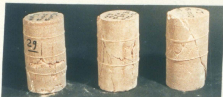
Plate 6.10 Natural shear surfaces established in intact PS specimens at zero (from left, 1&2) and 10 MPa (no. 3) confining pressure, and then tested as jointed specimens; confining pressure 30 MPa; type of loading, left to right, constant loading and straining, cyclic loading and constant loading and straining.
