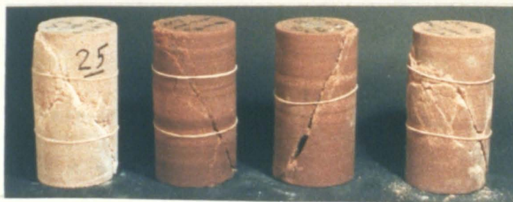
Plate 6.9 Natural shear surfaces established in intact PS specimens at zero (from left, 1 & 2) and 10 MPa (3 & 4) confining pressure, and then tested as jointed specimens, left to right, 70 MPa, multi-stage test, 70 MPa & multi-stage test.
