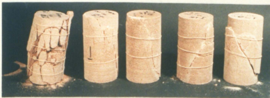
Plate 6.1 Fractured and deformed unjointed (intact) PS specimens, confining pressure, left to right, 0, 5, 10, 15, & 30 MPa.
