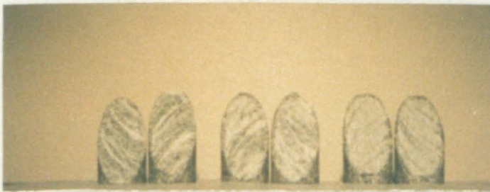
Plate 9.1: Sliding surfaces of granite specimens with saw cut joint after test, confining pressure left to right: 10, 30 & 70 MPa.
