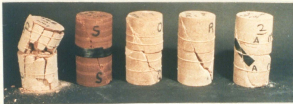
Plate 6.2 Fractured and deformed PS specimens with saw cut joint, confining pressure, left to right, 0, 5, 10, 15, & 30 MPa, joint angle=0°.
