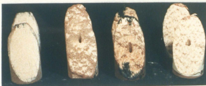
Plate 6.8 Natural and artificial joint sections after sliding and deforming along joint plane, joint angle = 60°, confining pressure, left to right, 15, 5, 15, & 30 MPa.
