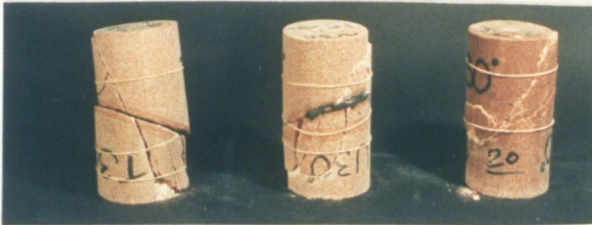
Plate 6.5 Fractured and deformed PS specimens with natural joint, confining pressure, left to right, 5, 15 & 30 MPa, joint angle = 30^\circ .
