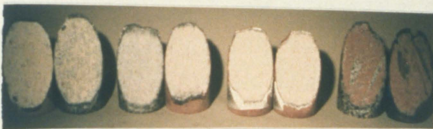
Plate 9.2 Sliding surfaces of combined rock types, left to right, limestone-granite, granite-sandstone, sandstone-sandstone, granite-slate, confining pressure= 70 MPa.
