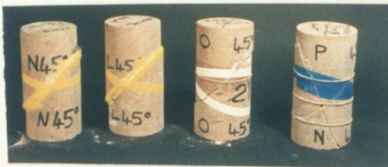
PLate 7.12 Fractured and deformed PS specimens under different loading and straining conditions, joint angle= 45^\circ , type of joint, left to right: natural (1 & 2) and saw cut (3 & 4), type of loading and straining: relaxation, constant strain and loading rate, cyclic loading, different strain rates (slow to fast); confining pressure, 15, 30, 30, & 15 MPa.
