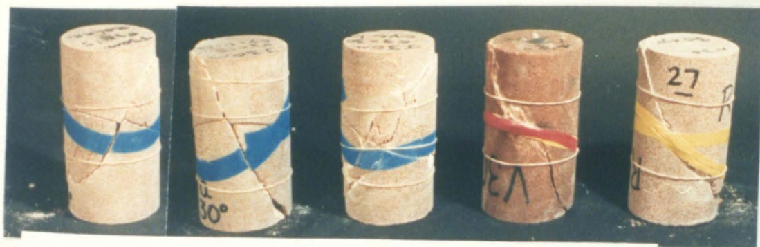
Plate 7.10 Fractured and deformed PS specimens under different loading conditions, joint angle= 30^\circ , type of loading: relaxation (no. 1) and cyclic loading (the rest), type of joint, left to right: saw cut (1 & 2 & 3) and natural (4 & 5), confining pressure, 15, 15, 30, 15 & 30 MPa.
