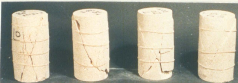
Plate 7.2 Fractured and deformed unjointed SS specimens, strain rate= 2.08 \times 10^{-6} , confining pressure, left to right, 0, 5, 10 & 15 MPa.
