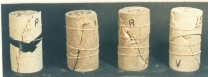
Plate 7.4 Fractured and deformed SS specimens, joint angle= 30^\circ , strain rate= 8.33 \times 10^{-4} , confining pressure, left to right, 0, 5, 10 & 15 MPa.
