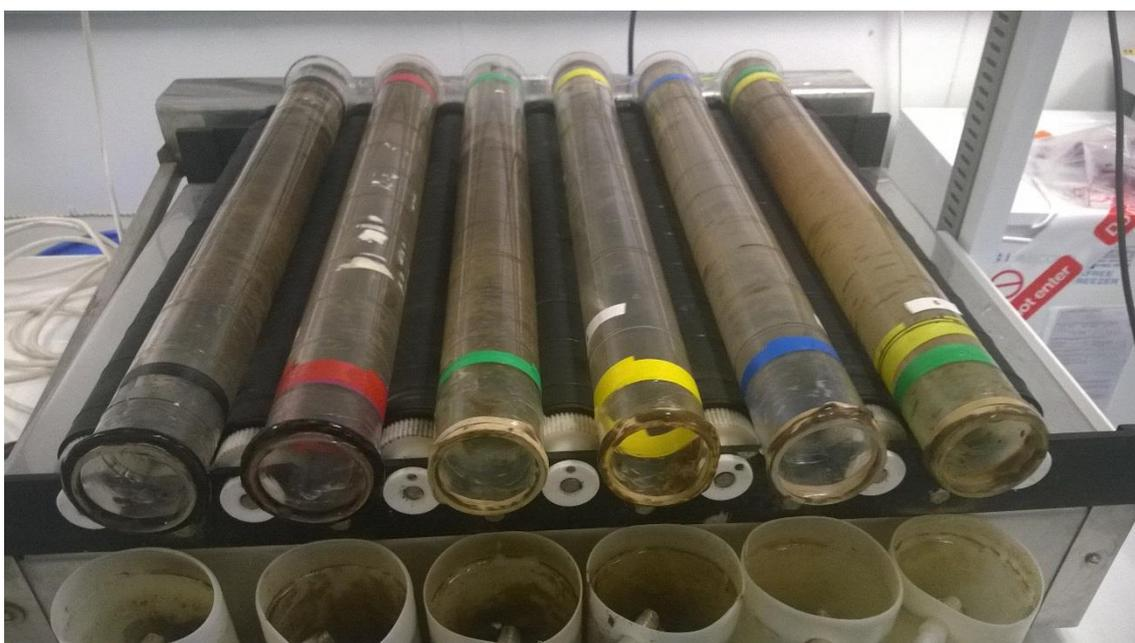
*Figure 5-3 Photo of the six rotating tubular reactors, inclined at an angle of approximately one degree to the horizontal. Starting from the left the reactor amendments were as follows: Control (R1; black label), 2.00 meropenem (R2, red label), 2.00 Zn (R3; green label), 2.00 mg/L meropenem and 2.00 mg/L Zn (R4; yellow label), 2.00 mg/L meropenem and 20.0 mg/L Zn (R5; blue label), 2.00 mg/L meropenem and 100 mg/L Zn (R6; yellow/green label).*
