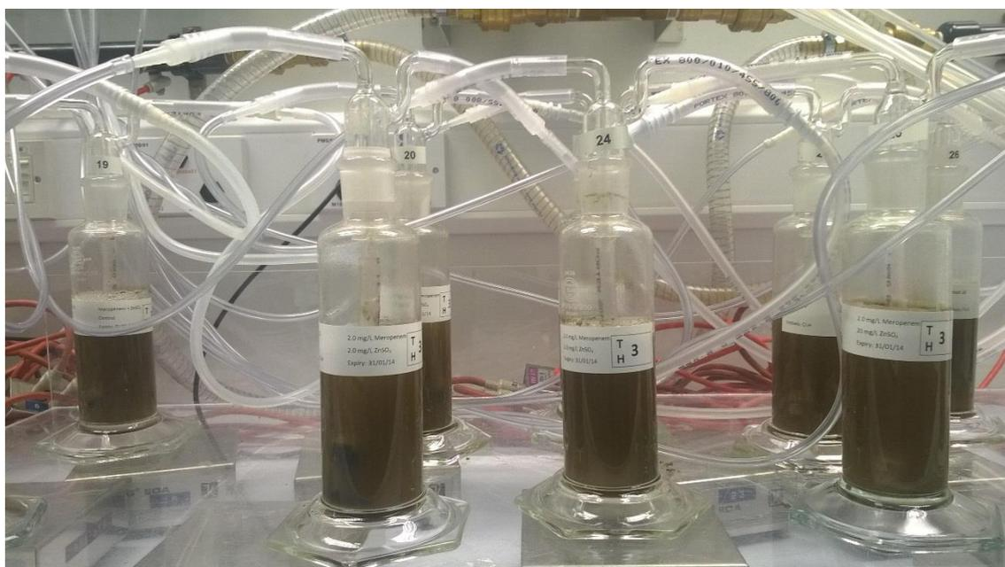
*Figure 5-2 Photo of the set-up of aerated glass test vessels used for the definitive ASRIT study, with the appropriate meropenem and Zn amendments, activated sludge at a sludge solids concentration of 1.50 g/L, 5.00 ml of synthetic sewage feed and, de-ionised water to give a total volume of 150 ml.*
