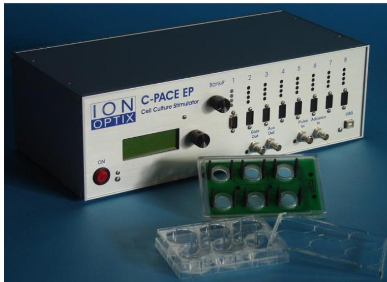
Figure 4.5: EPS was performed using the C-pace EP cell pacer (Ion Optix, Dublin)
