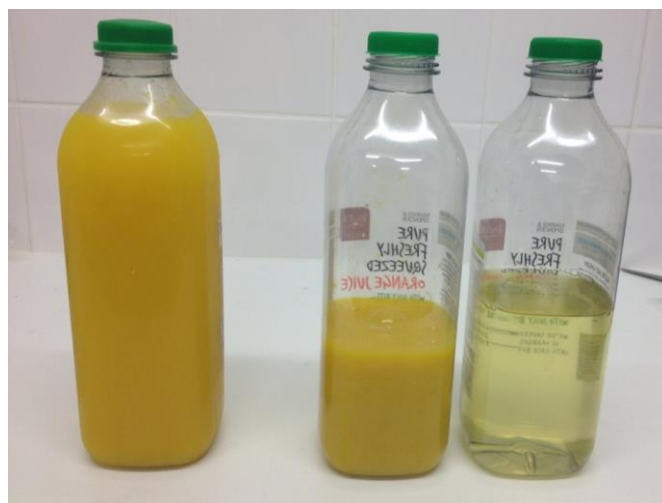
Figure 4.58. Fresh juice (at the left) the filtrate (at the right), and the blended concentrate (in the middle) at the end of the experiment (normal orientation, 30V, 4bar, 0.2 \mu filtrate and 5.5hr duration)
