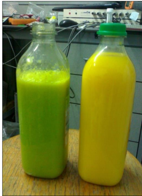
Figure 3.13. Orange juice before and after the electrokinetic treatment with copper electrodes
