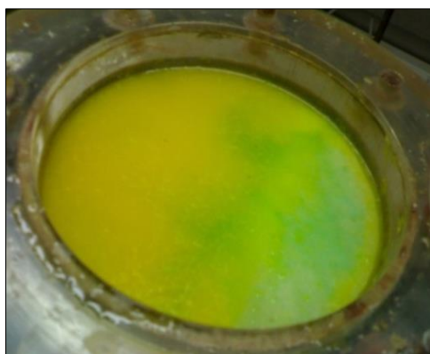
Figure 3.12. Blue-green copper salt in juice at the electrode interface
