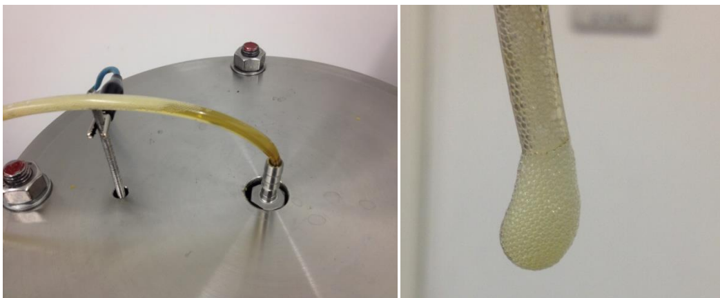
Figure 4.33. The bubbles clusters flow out from the top outlet
