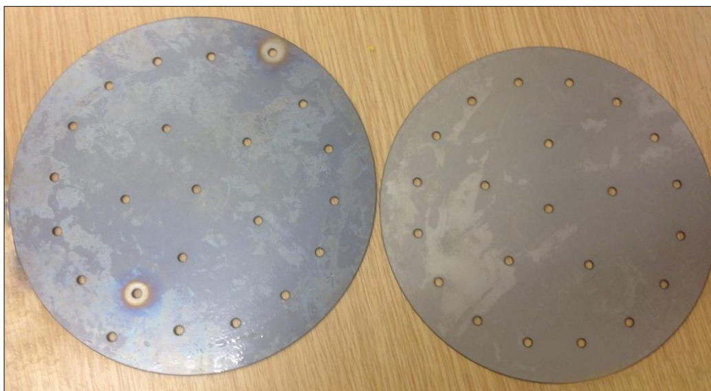
Figure 3.14. Perforated Titanium disc as electrode
