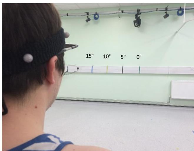
**Figure 4-5 – Photograph of electro-oculography (EOG) calibration procedure; lines on the wall represent the targets set at 5°, 10° and 15°**
