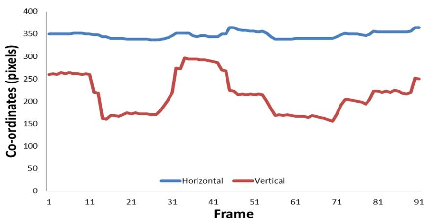
**Figure 5-1 - Example raw data from Dikablis mobile eye-tracker during walking**
