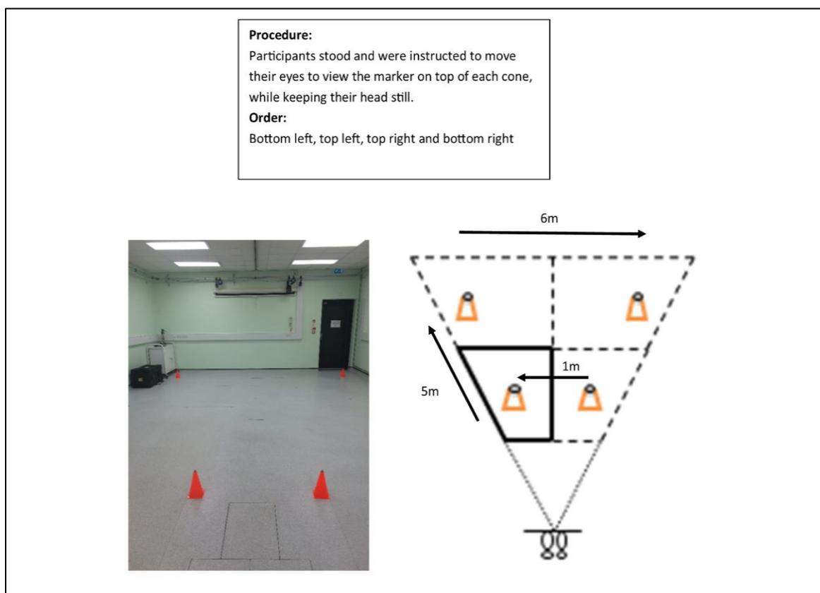
**Figure 4-4- Mobile eye-tracker calibration procedure**
