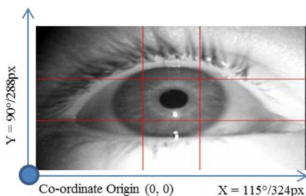
**Figure 5-2 – Eye-view camera alignment and co-ordinates (px = pixels)**
