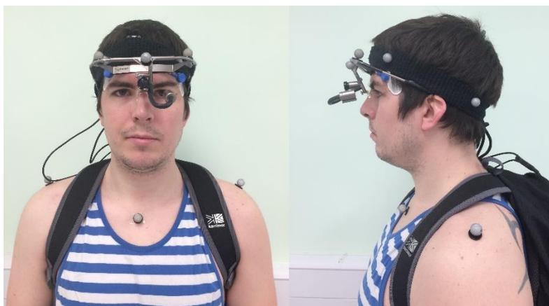
**Figure 4-3- Mobile eye-tracker and EOG placement**
