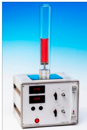
Figure 1.4: view of LOI apparatus. Photograph taken from FTT website
