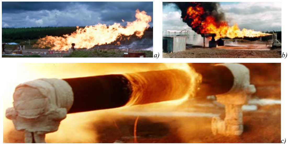
Figure 1.10: Jet fire tests in progress: a) from Hydrocarbon Processing; b) from DNV websites; c) impact of the flame on a full scale steel pipe with fire protection
