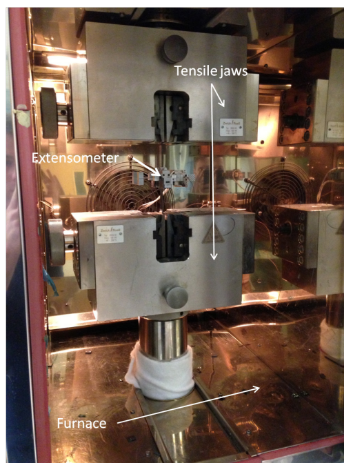
Figure 3.3: Tensile testing jaws enclosed in the furnace, picture taken at Cytec premises, Heanor, UK.
