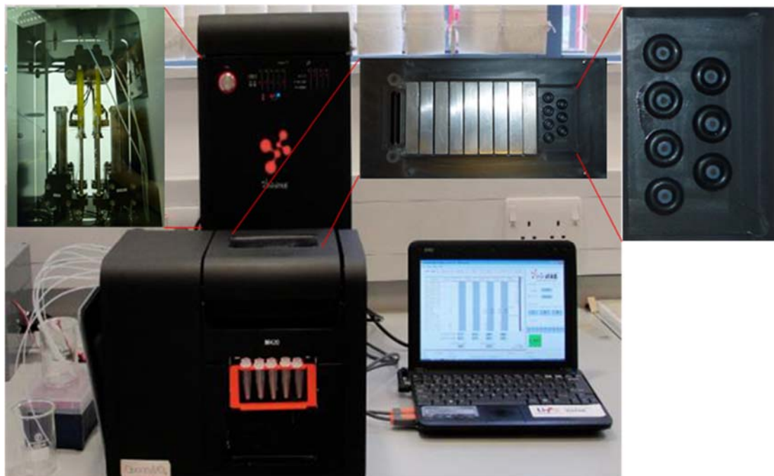
Figure 2.2: The QuantuMDx prototype (The MiniChemLab) with the cassette manifold (right corner) and the syringe pumps (left corner).
