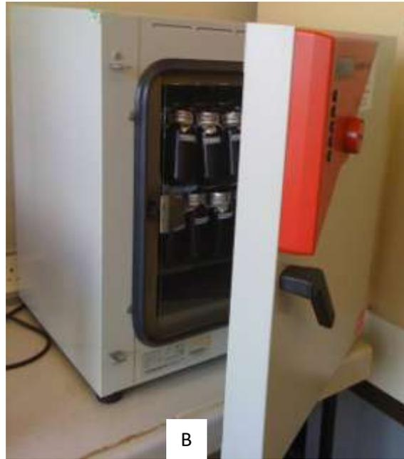
Figure 3.3: Sample bottles containing compost mixes in (A) E-class Max Q400 shaker incubator and (B) Binder BF53 incubator with forced convection
