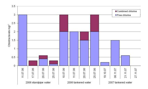
Figure 6.2: Chlorine levels in standpipe samples and tankered source samples
