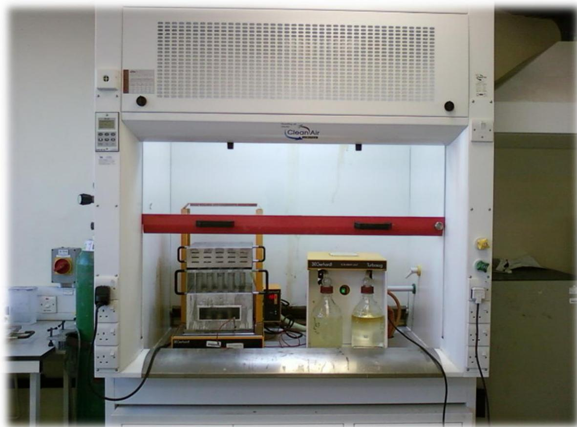
**Plate 3.4 Digestion chamber for fibre determination**
