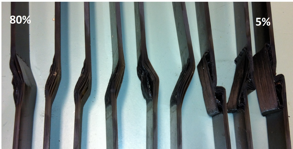
Figure 7.13: Effect of reduction in applied load levels (from left to right) on failure characteristics of unprotected CFRP specimens tested under compressive loading while under exposure to one sided heating of 50 \text{ kW m}^{-2} .
