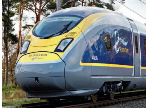
Figure 1.3: Composite nose design in Siemens Velaro train family used as Eurostar, ICE3, AVE or CRH3 [18].
