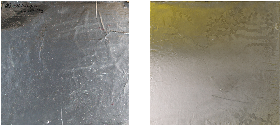
Figure 3.2: Fabricated PML a) before and b) after revision of manufacturing process.
