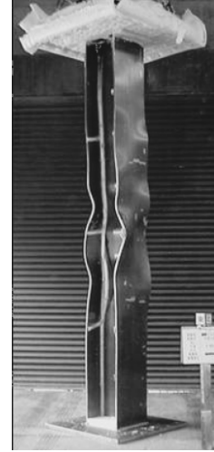
Figure 2.2: Deformed H-column specimen after structurally loaded heating test. Reproduced from [55].
