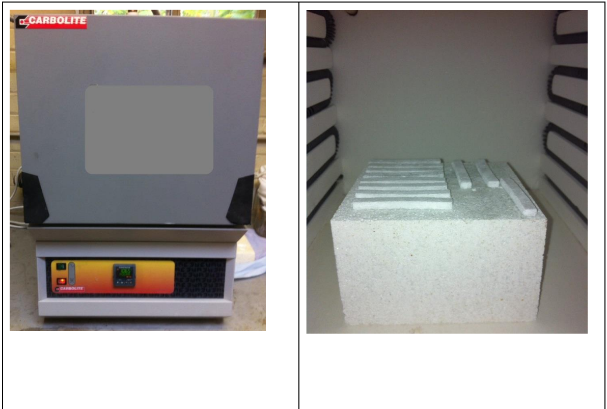
Figure 3.10 chamber furnace used for sintering AW green Parts
