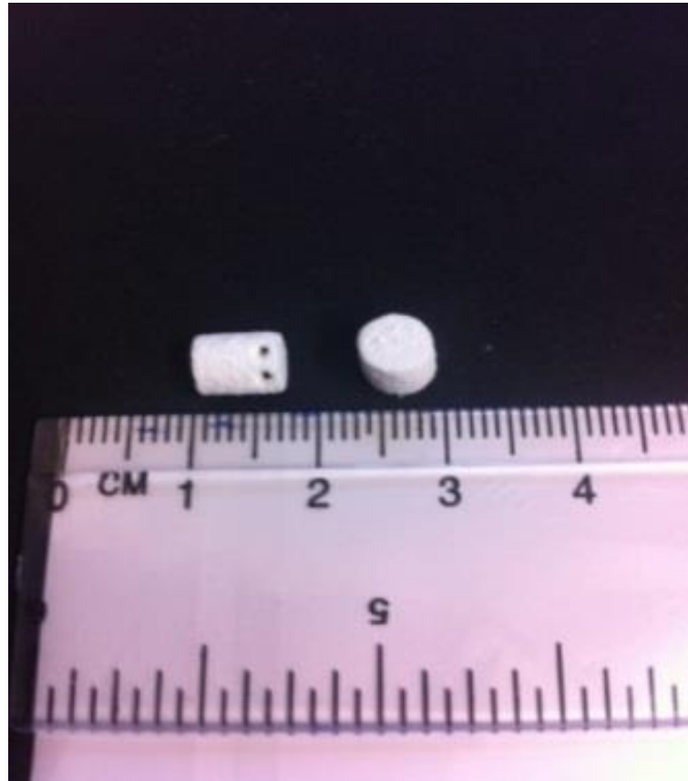
Figure 5.11 Printed and sintered plugs with two through holes of PB5
