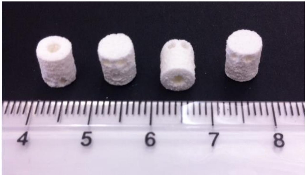
Figure 5.13 Printed and sintered plugs with two through holes and one pocket hole of PB5
