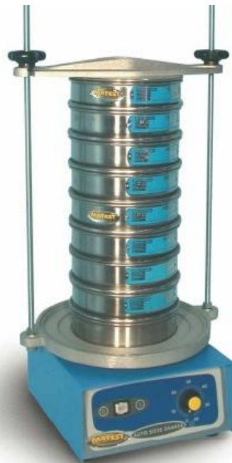
Figure 3.5 The sieve shaker used to give a range of particle sizes of AW and maltodextrin
