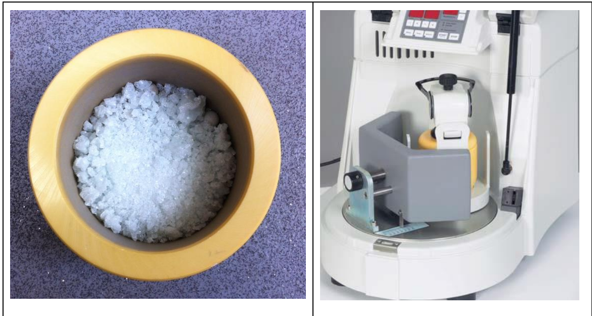
Figure 3.4 The ball mill used to grind the A-W and maltodextrin into powders
