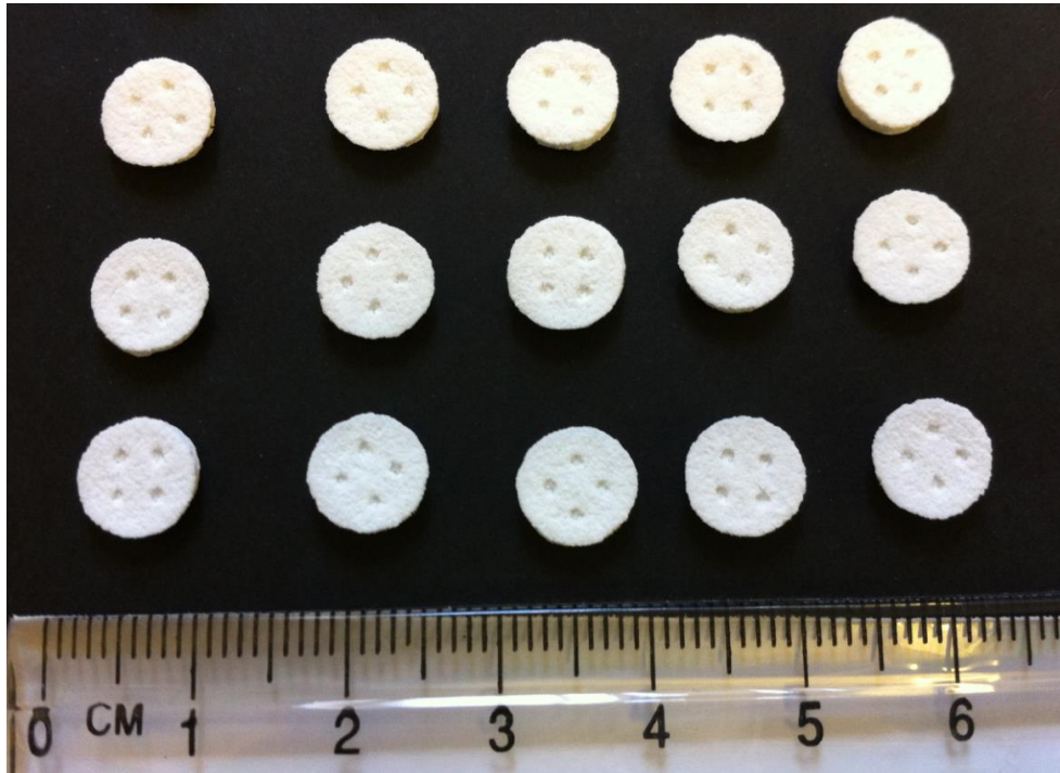
Figure 5.7 Printed and sintered discs with four pockets of PB1
