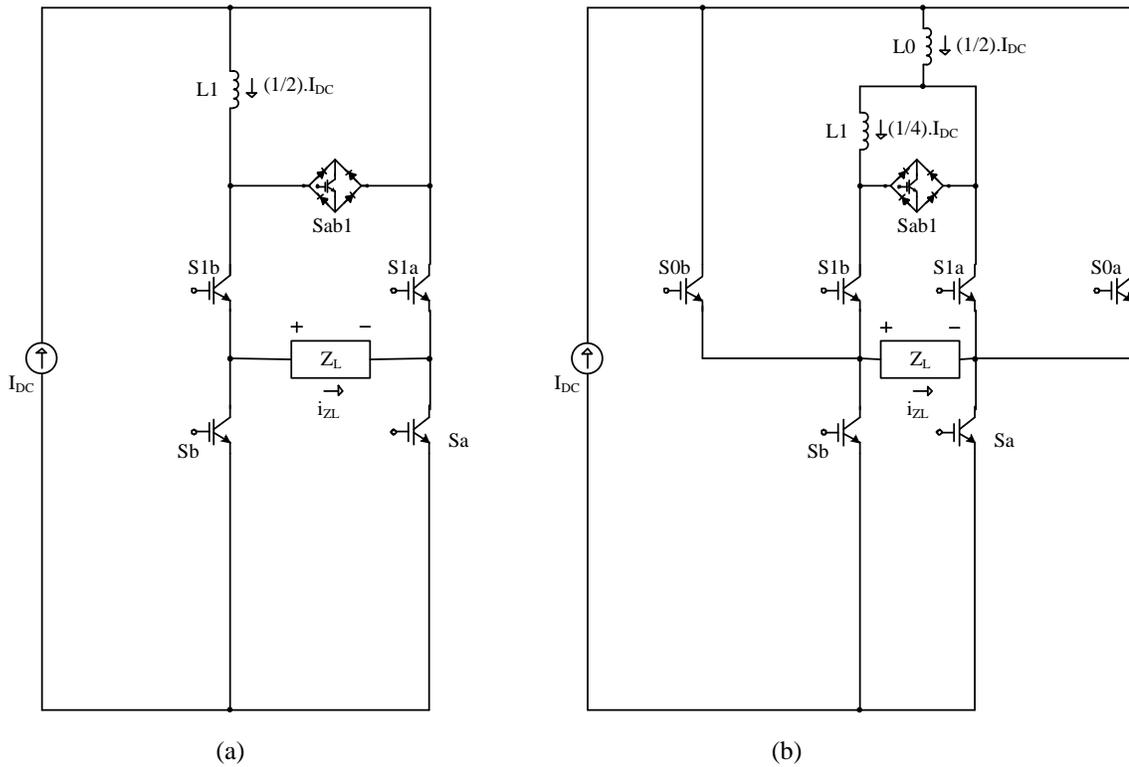
Fig.4 - 3: (a) The novel 5-level CSI (b) The novel 9-level CSI
