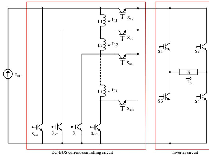
Fig.2 - 27: Generalized structure of Topology III
