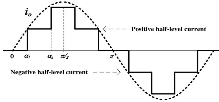
Fig.3 - 5: Quarter wave symmetrical five-level output current
