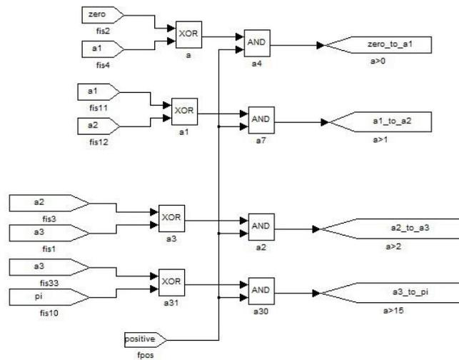
Fig. A.6: The positive cycle block
