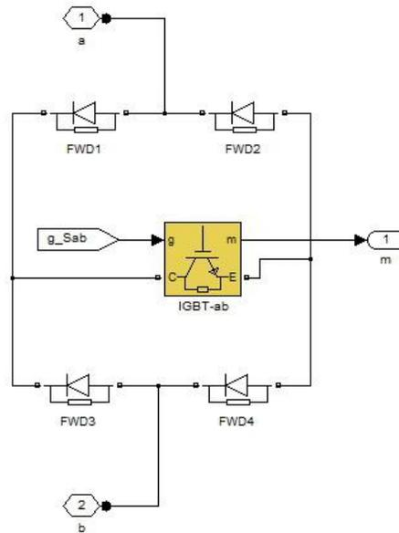
Fig. A.2: The bidirectional IGBT switch
