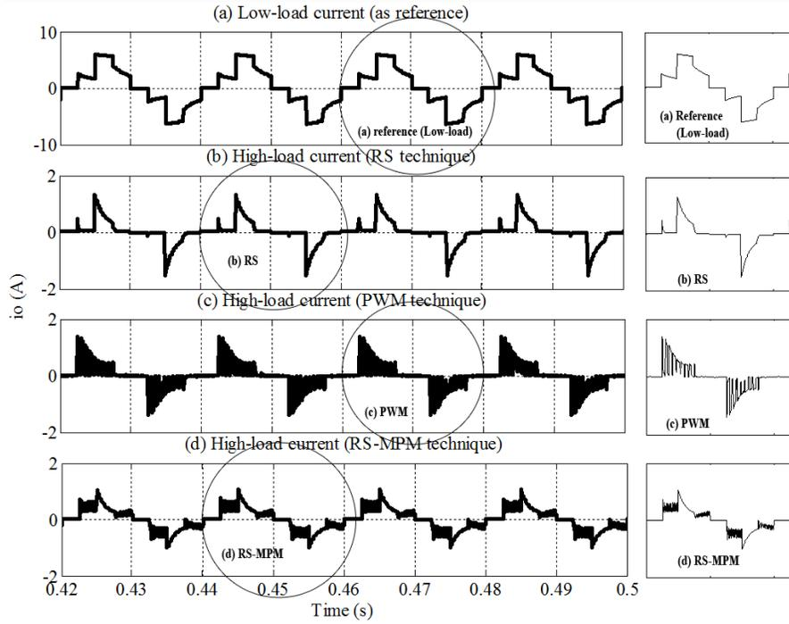
Fig.3 - 11: Simulated output current waveforms; high resistive load (from the top: low-load current for reference, RS, PWM and RS-MPM)
