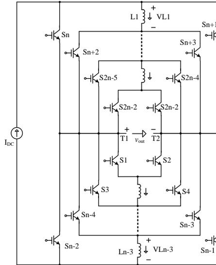
Fig.1 - 2: The generalized structure of Topology I
