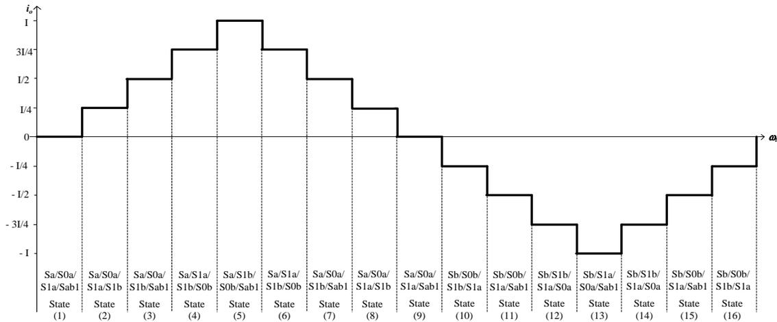
Fig.4 - 6: Nine-level CSI switching sequence
