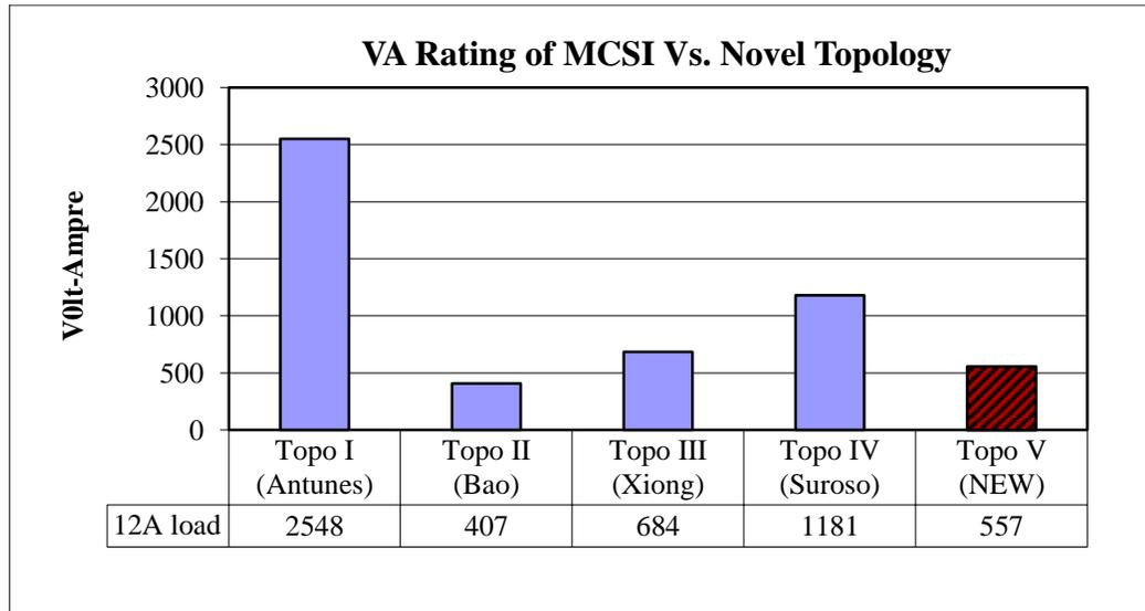
Fig.4 - 17: VA rating of novel topology
