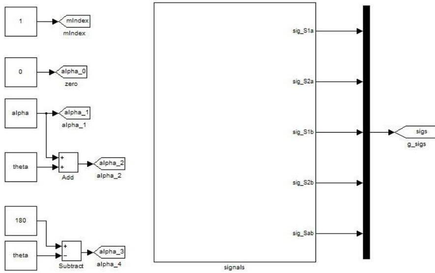
Fig. A.3: The gate signal blocks
