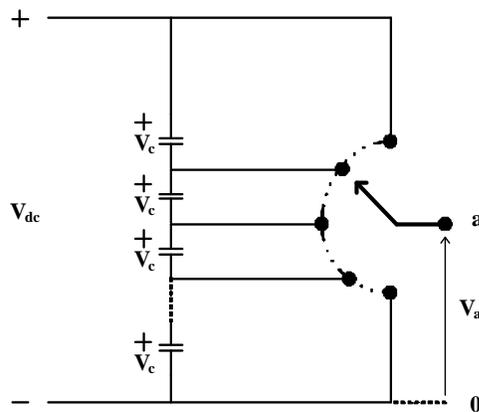
Fig.2 - 4: Multilevel inverter fundamental
