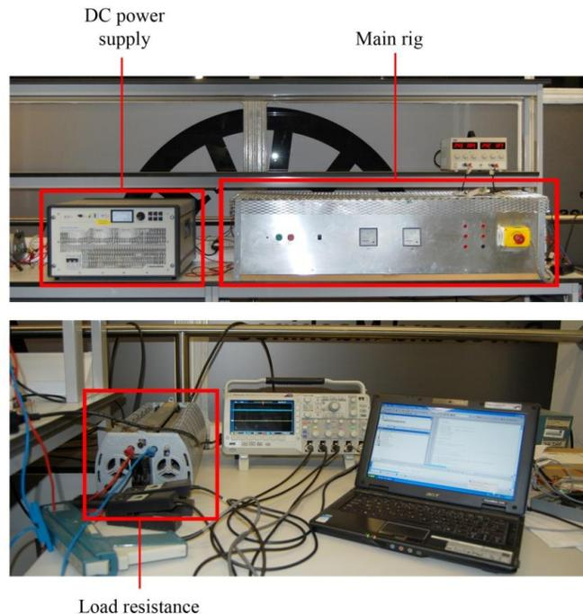
Fig.5 - 7: Complete MCSI experimental arrangement set-up
