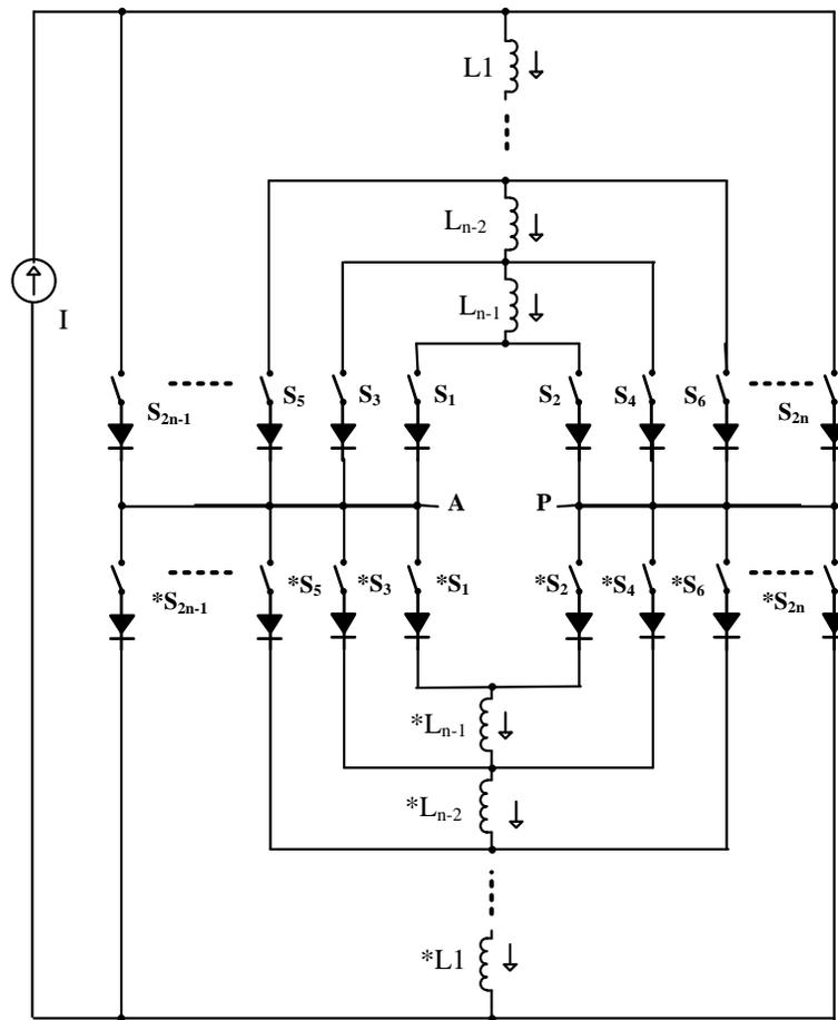
Fig.2 - 16: Final MCSI circuit
