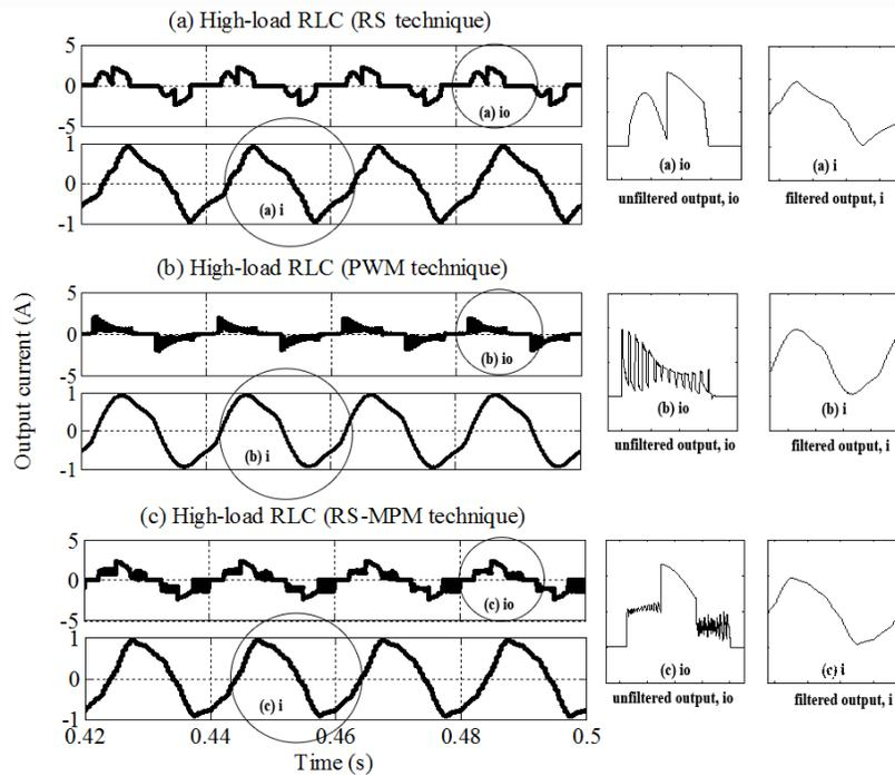
Fig.3 - 12: Simulated output current waveforms ( $i_o$  &  $i$ ); high RLC load
