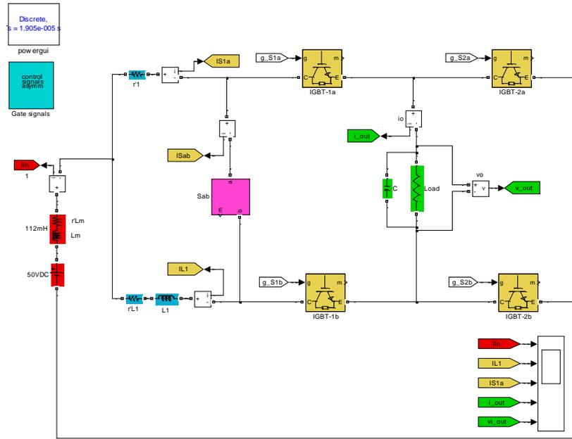
Fig.4 - 8: Matlab/Simulink model of the novel five-level CSI
