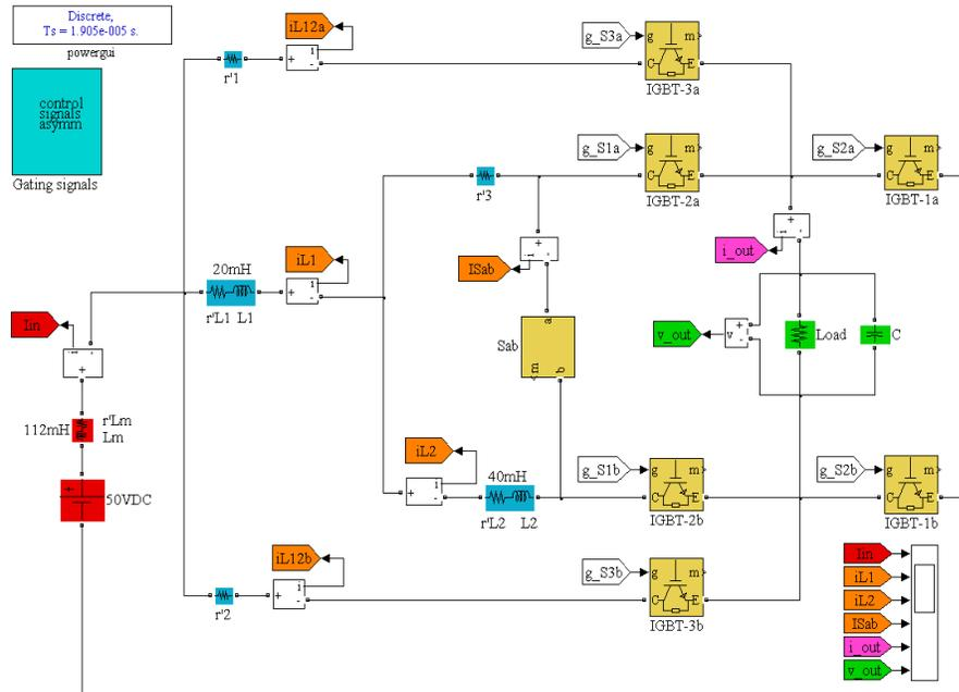
Fig.4 - 9: Matlab/Simulink model of the novel nine-level CSI
