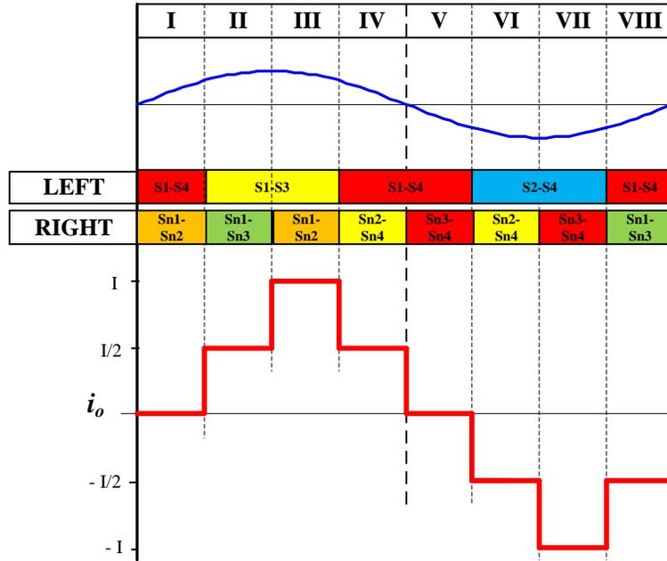
Fig.2 - 33: Topology IV five-level switching sequence
