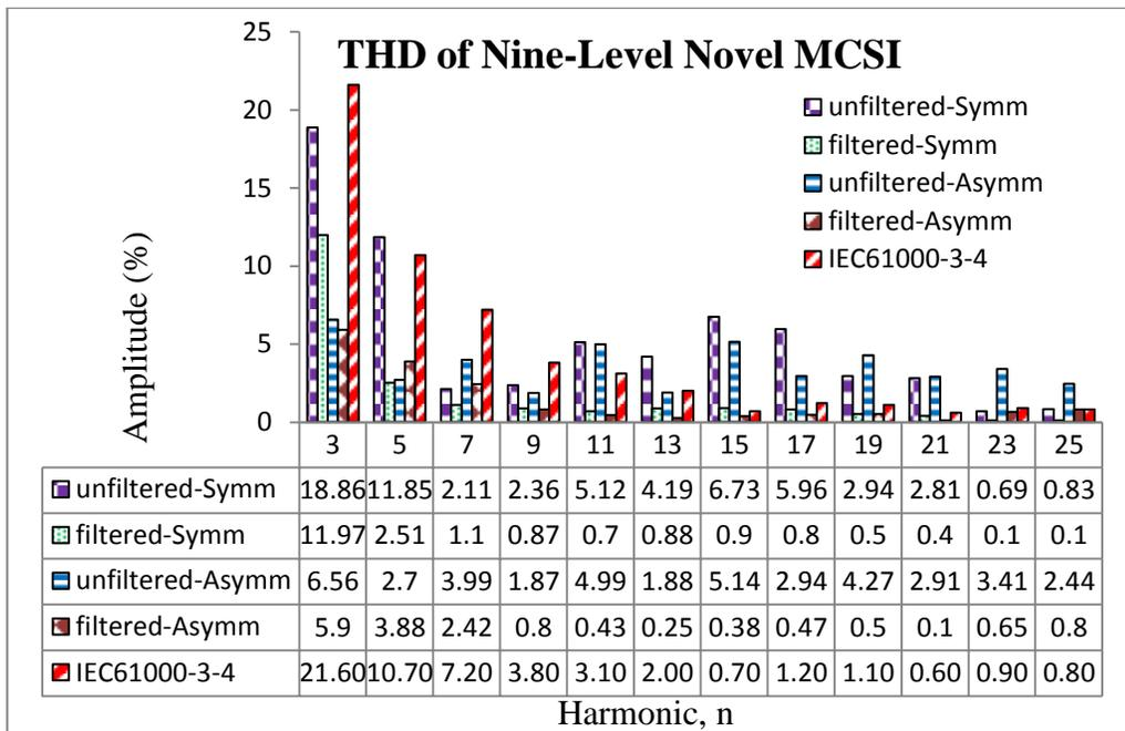
Fig.4 - 16: Current harmonic contents of the novel nine-level topology
