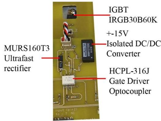
Fig.5 - 4: Single 316J driver circuit and IGBT
