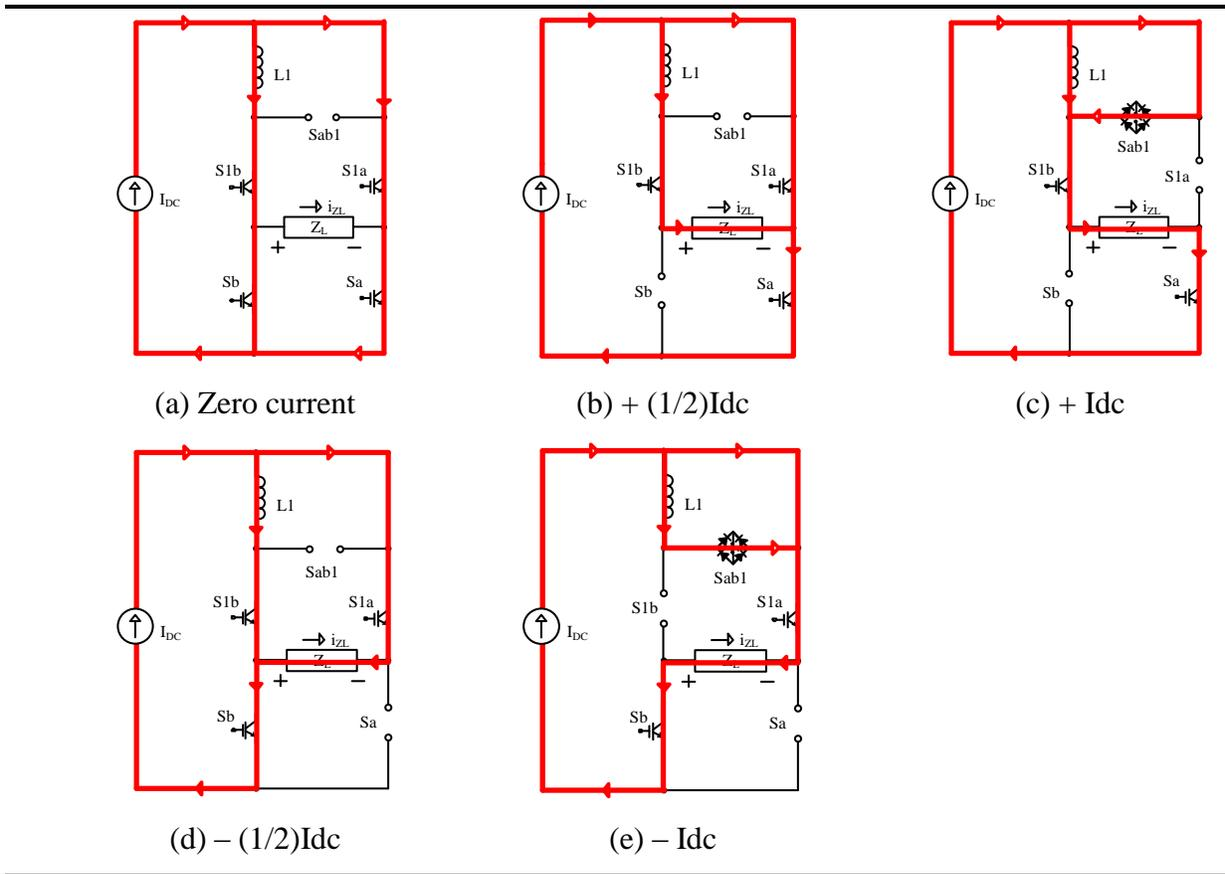
Fig.4 - 5: Load current path of the five-level CSI
