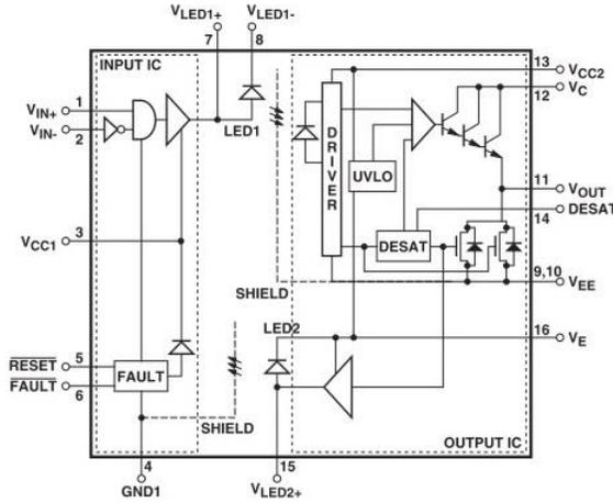
Fig.C.3: HCPL-316J IC inside components [99]
