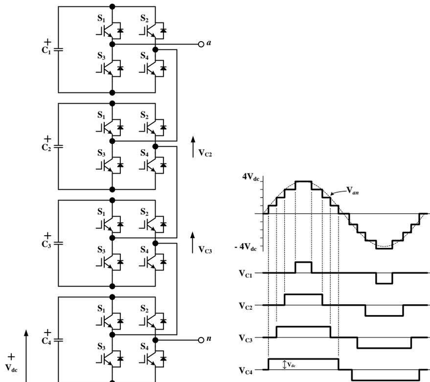
Fig.2 - 8: Cascaded inverter with corresponding output waveform
