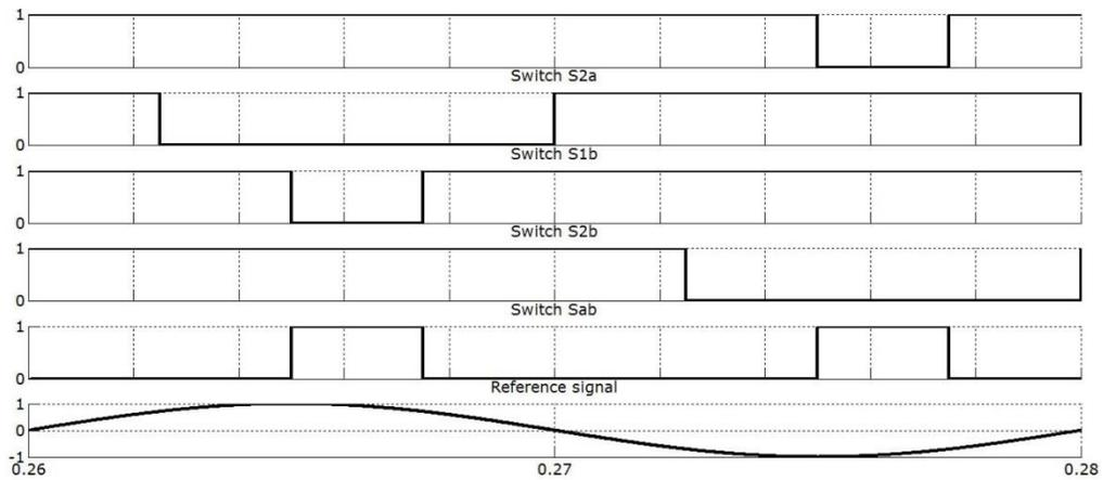
Fig. A.5: The control signals
