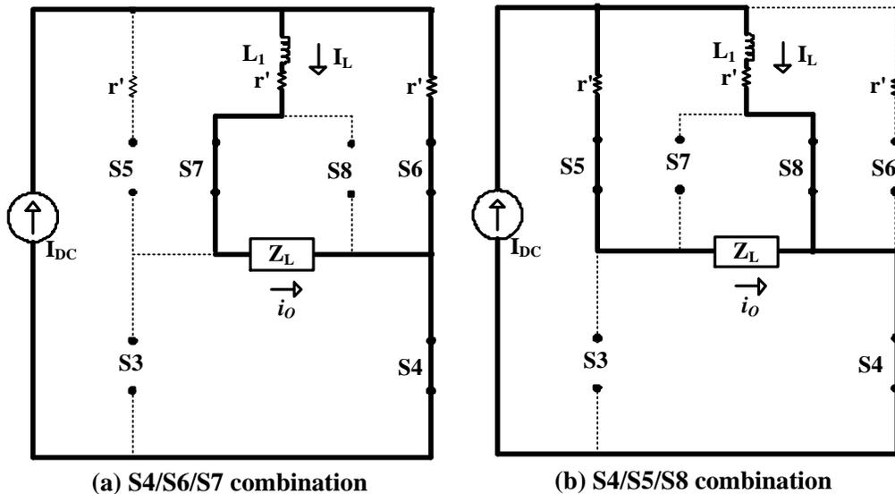
Fig.3 - 7: Half-current redundant switching states
