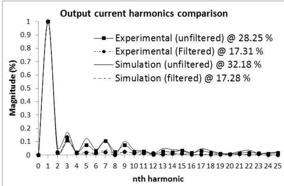
Fig.5 - 14: Harmonics comparison between experimental and simulation
