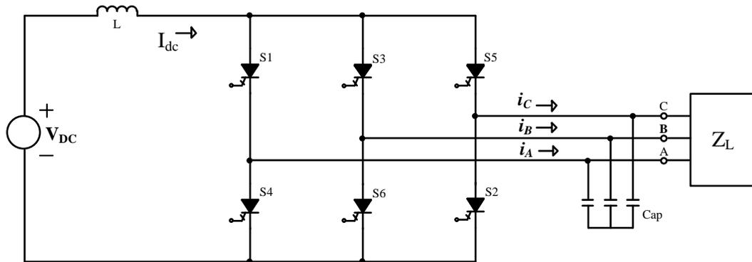
Fig.2 - 9: Schematic of a classical SCR-based CSI
