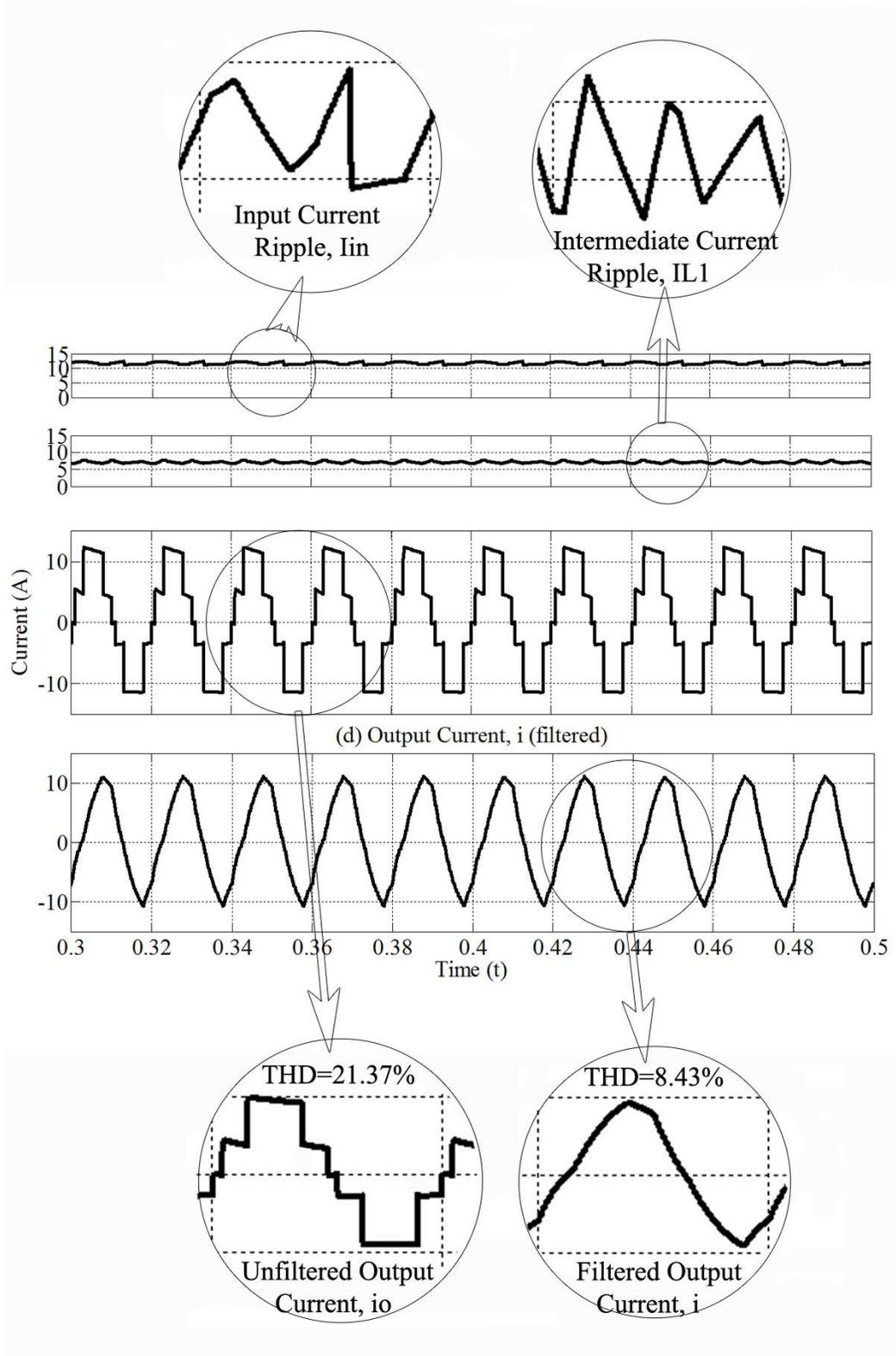
Fig.4 - 12: Five-level CSI with selected switching angles
