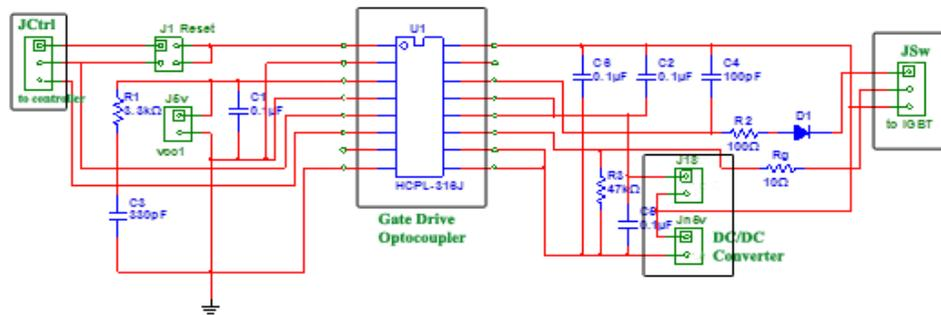
Fig.C.4: Schematic for the gate driver circuit
