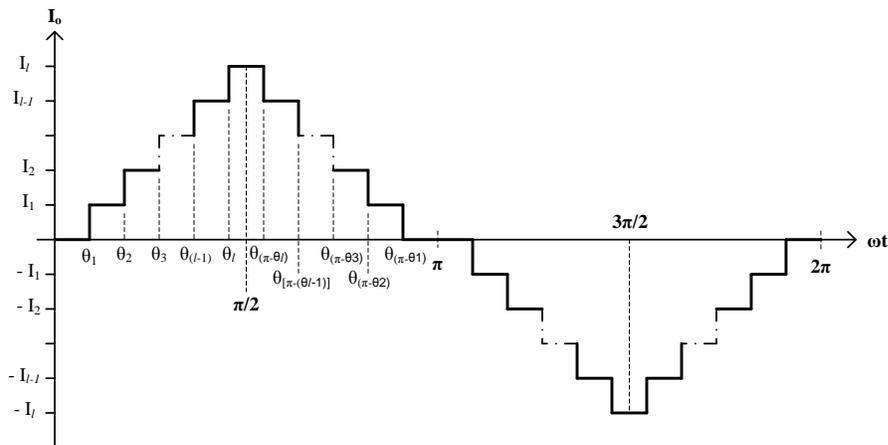
Fig.2 - 2: Output current waveform of a general single-source MCSI
