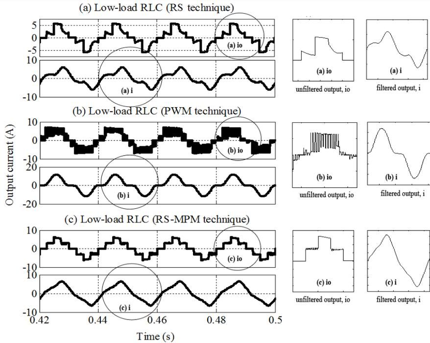
Fig.3 - 10: Simulated output current waveforms ( $i_o$  &  $i$ ); low RLC load
