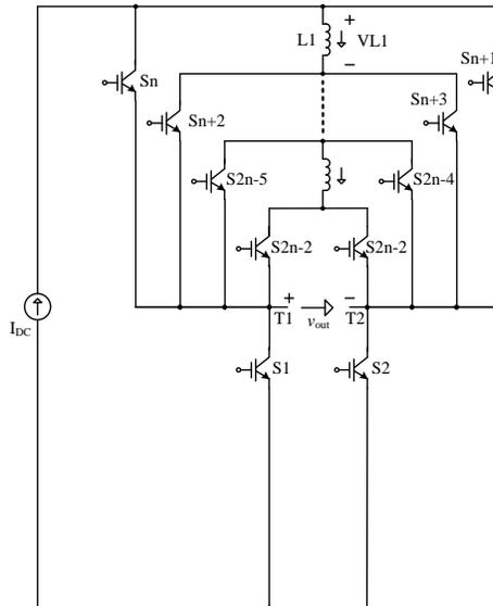
Fig.1 - 3: The generalized structure of Topology II
