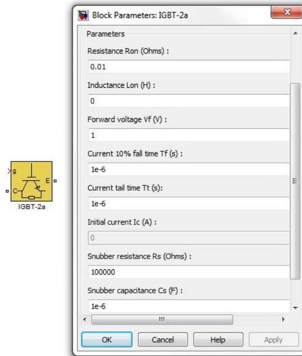
Fig.A.1: The IGBT block showing the dialog box and parameters
