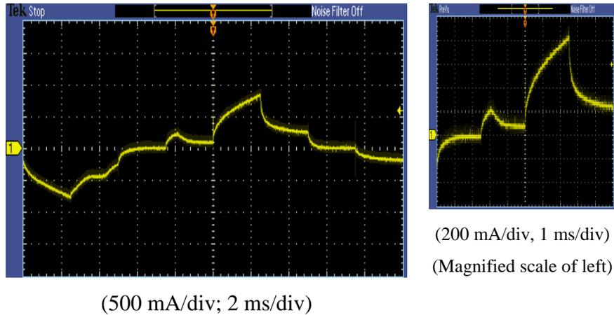
Fig.3 - 15: Five-level output current at high-load condition (with RS technique)
