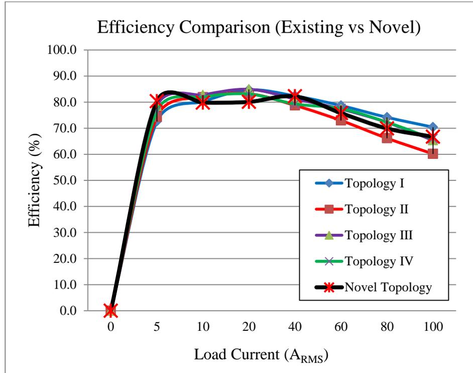
Fig.4 - 18: Efficiency vs. Load current of novel topology
