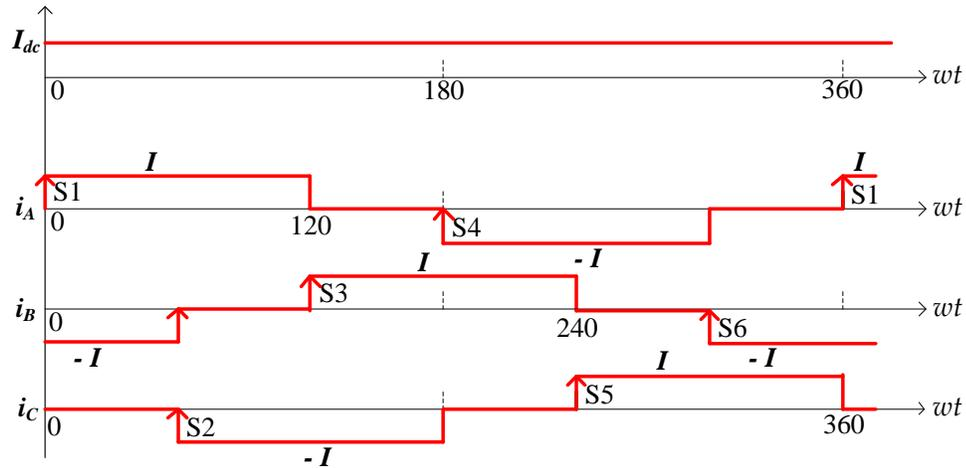
Fig.2 - 10: Three-phase SCR-based CSI typical current waveforms
