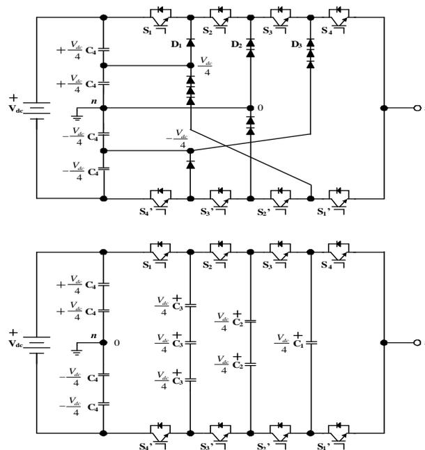
Fig.2 - 7: Re-drawn figures of the (top) five-level diode-clamped inverter and (bottom) capacitor-clamped inverter
