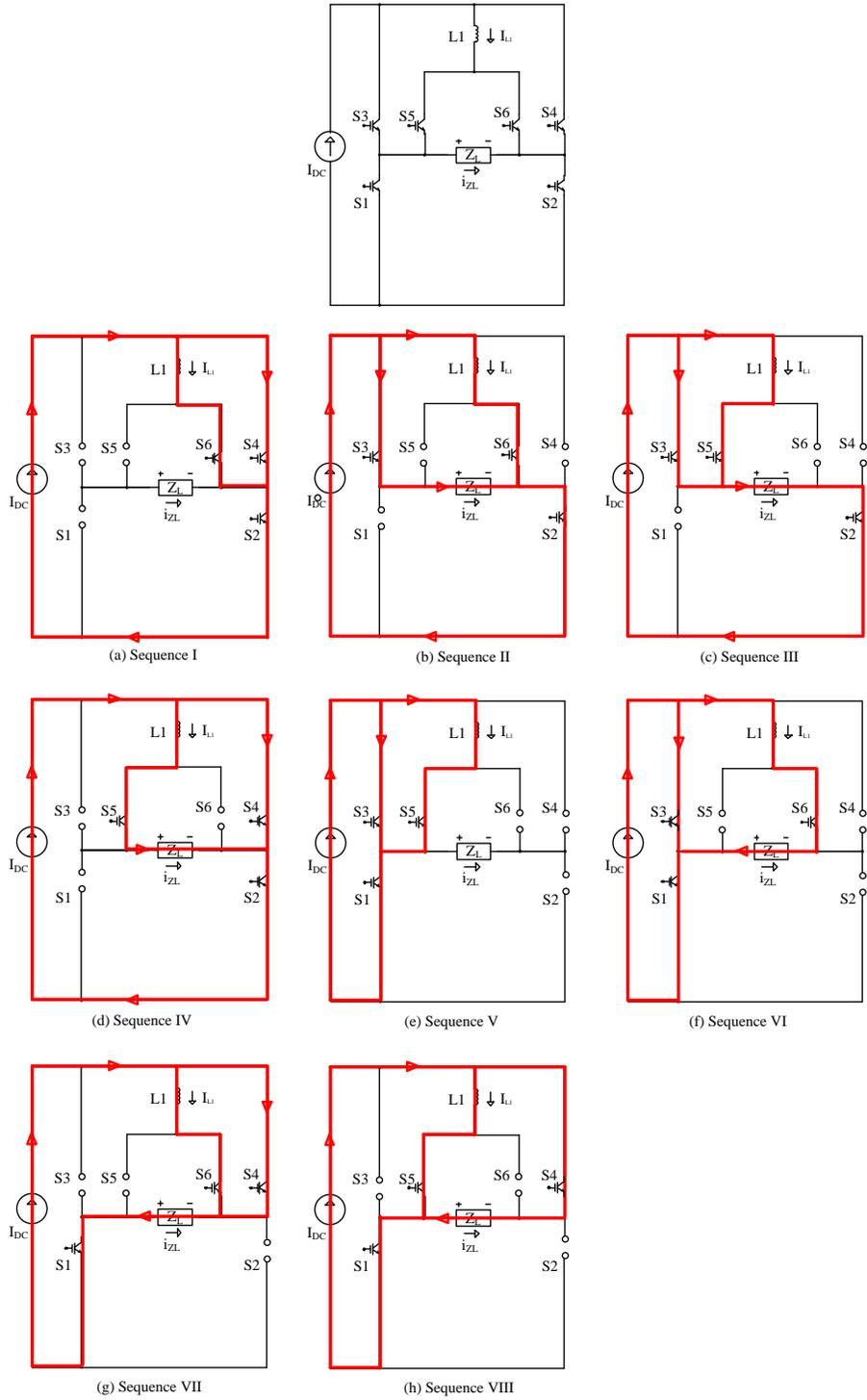
Fig.2 - 26: Single-phase five-level inverter circuit and its corresponding switching sequences (a)-(h)
