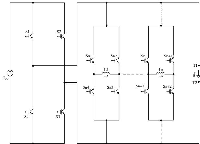
Fig.1 - 5: Generalized structure of Topology IV
