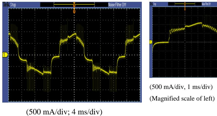
Fig.3 - 16: Improved output current at high-load condition (with RS-MPM)
