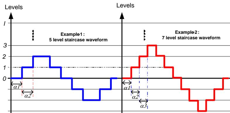
Fig.2 - 1: Converter output level determination
