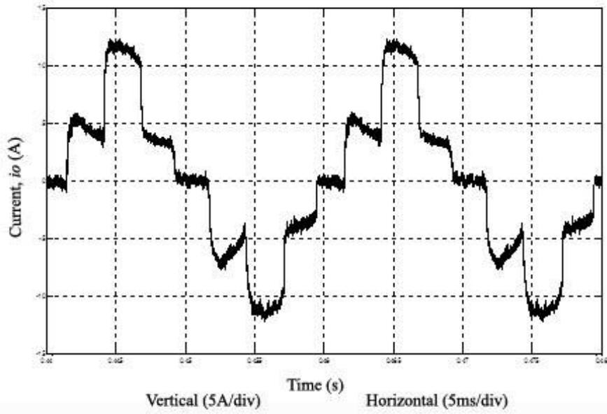
Fig.5 - 9: The five-level output current waveform
