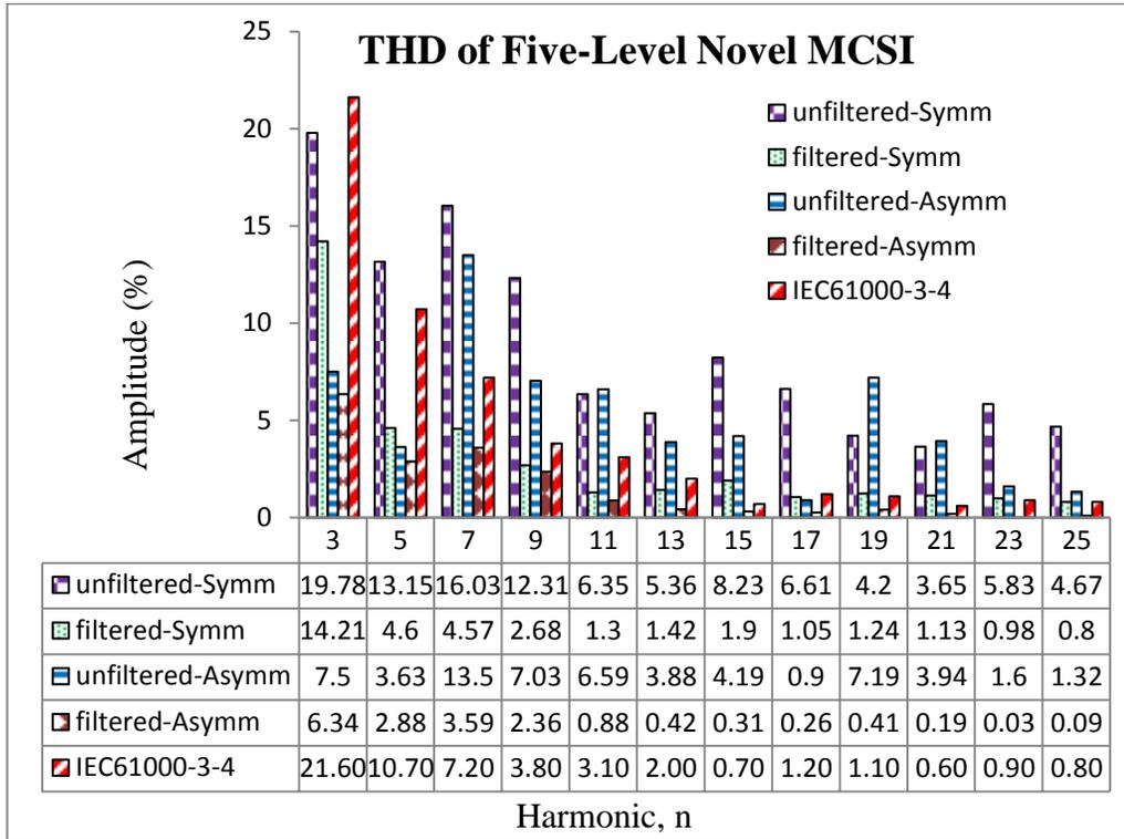
Fig.4 - 15: Current harmonic contents of the novel five-level topology
