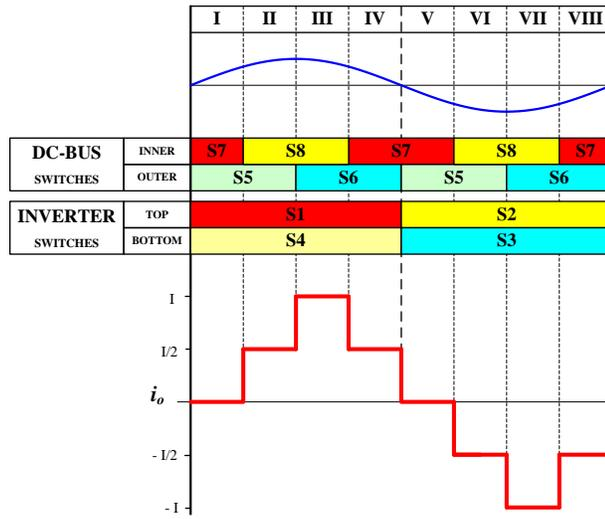
Fig.2 - 29: Topology III Five-level switching sequence
