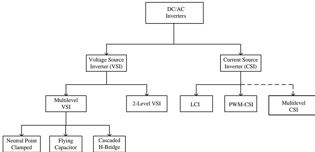
*Fig.1 - 1: General Classification of Inverters*
