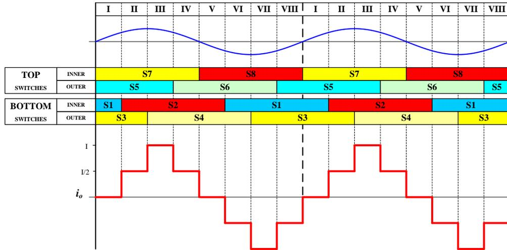
Fig.2 - 21: Five-level symmetric switching sequence
