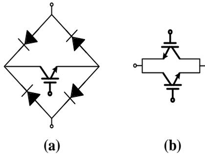
Fig.4 - 1: (a) 1-IGBT with 4-diodes (b) 2-IGBTs in parallel
