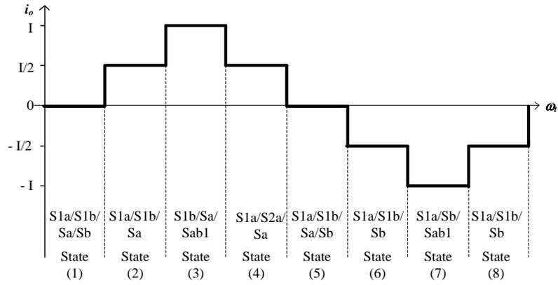
Fig.4 - 4: Five-level CSI switching sequence
