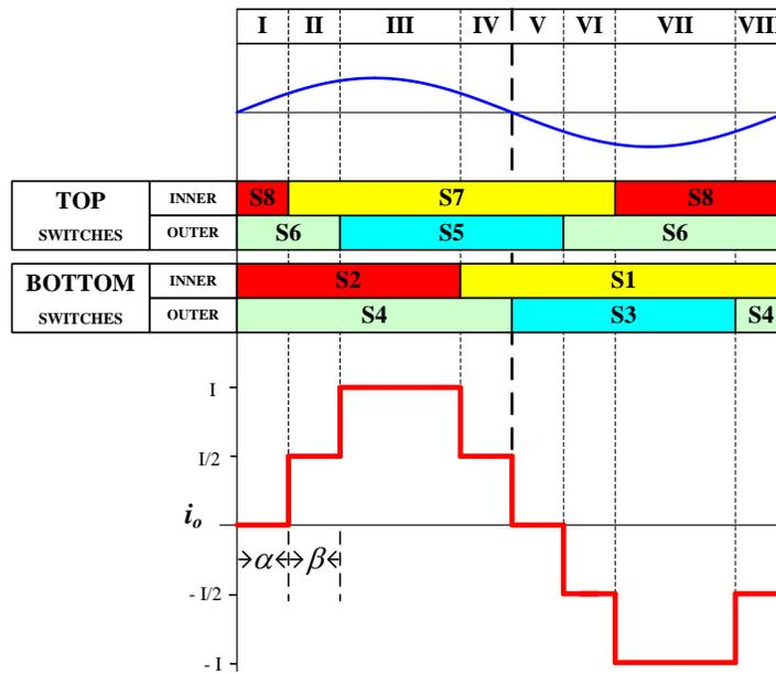
Fig.2 - 22: Five-level asymmetric switching sequence
