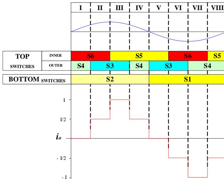
Fig.2 - 25: Topology II five-level switching sequence
