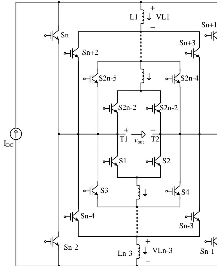
Fig.2 - 17: The generalized structure of Topology I
