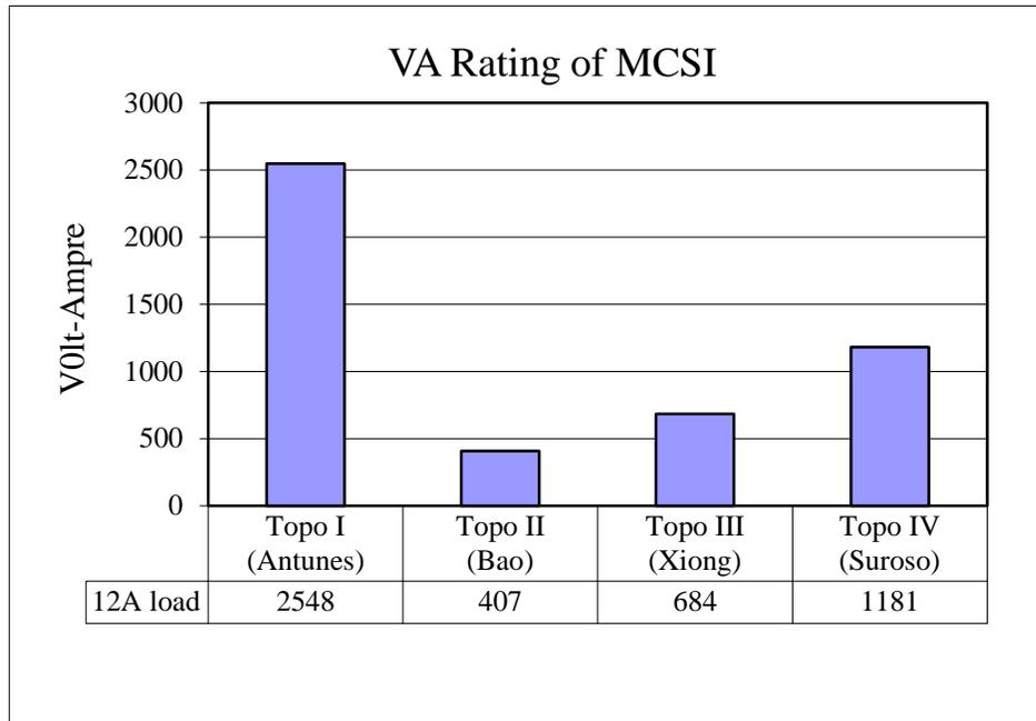
Fig.2 - 35: Volt-Ampere (VA) comparison
