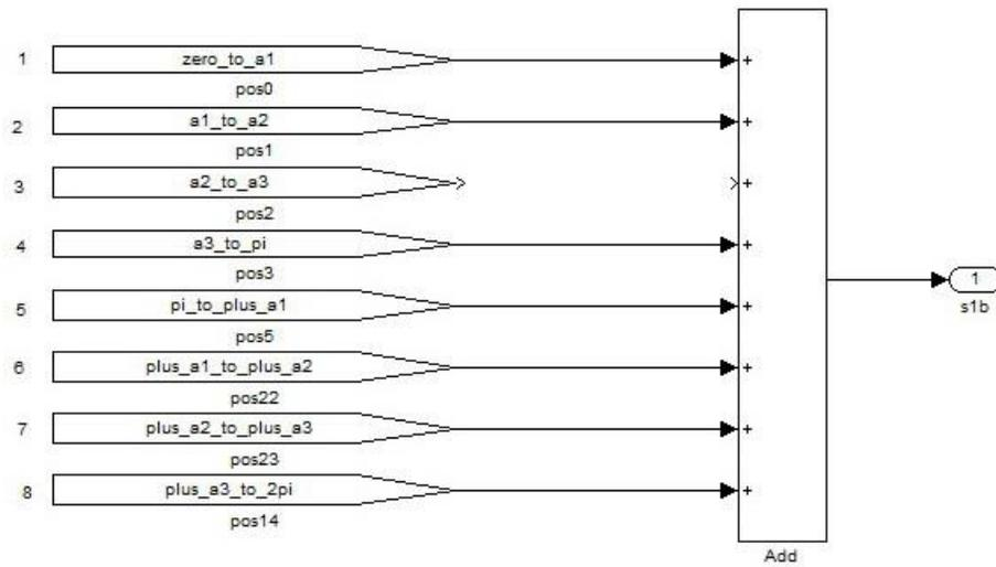
Fig. A.16: The logic signals of the switch S1b
