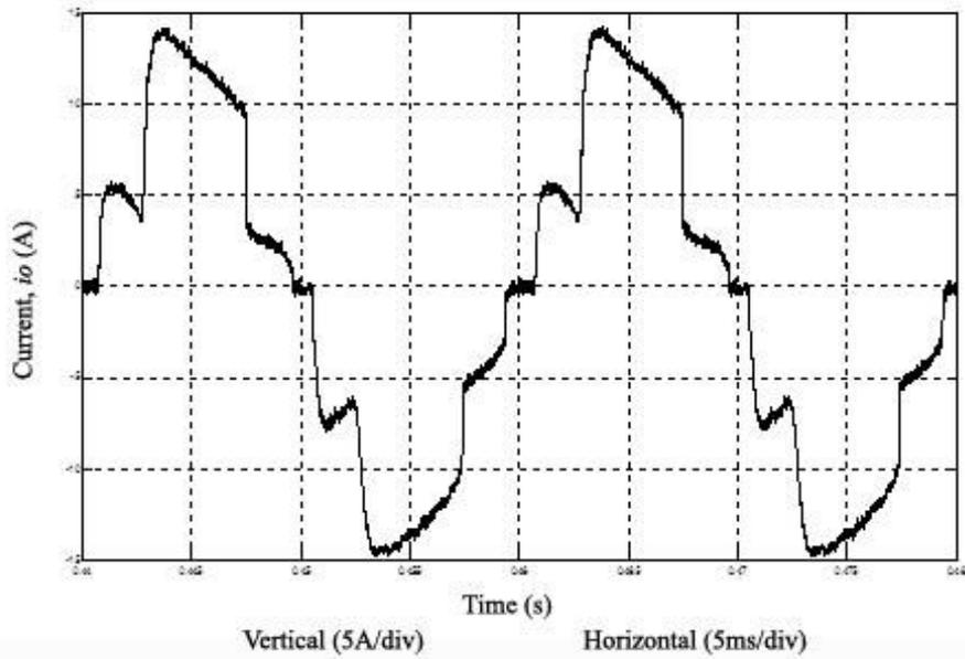
Fig.5 - 15: The five-level output current with different switching angles
