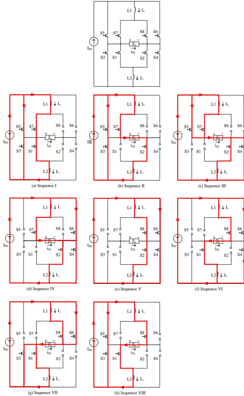
Fig.2 - 20: Single-phase five-level inverter circuit and its corresponding switching sequences (a)-(h)
