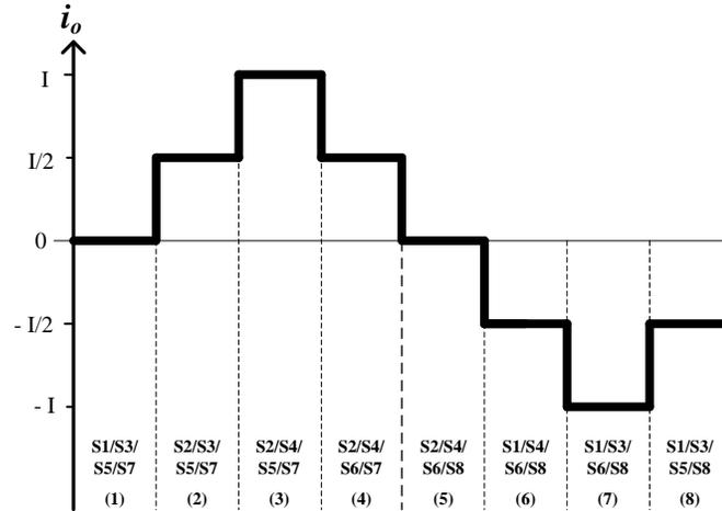
Fig.2 - 19: Five-level CSI switching sequence
