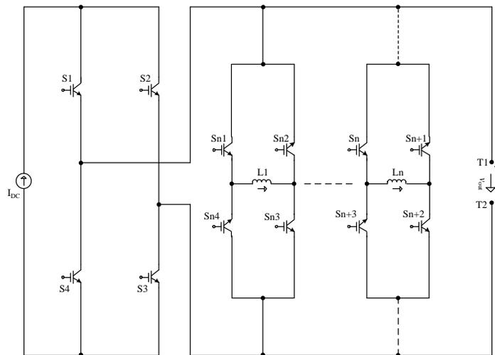
Fig.2 - 31: The generalized structure of the Topology IV
