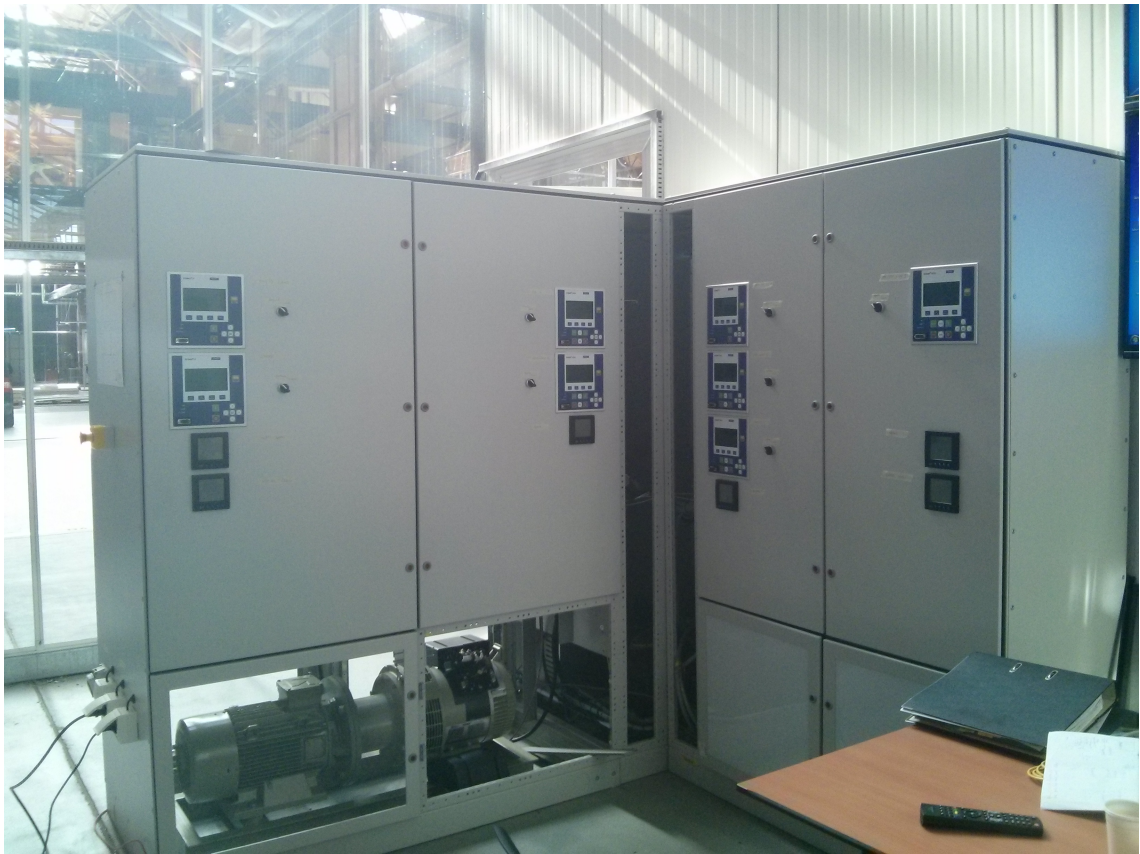
(a) Left hand side cabinet showing emulated diesel generator motor/generator pair.
