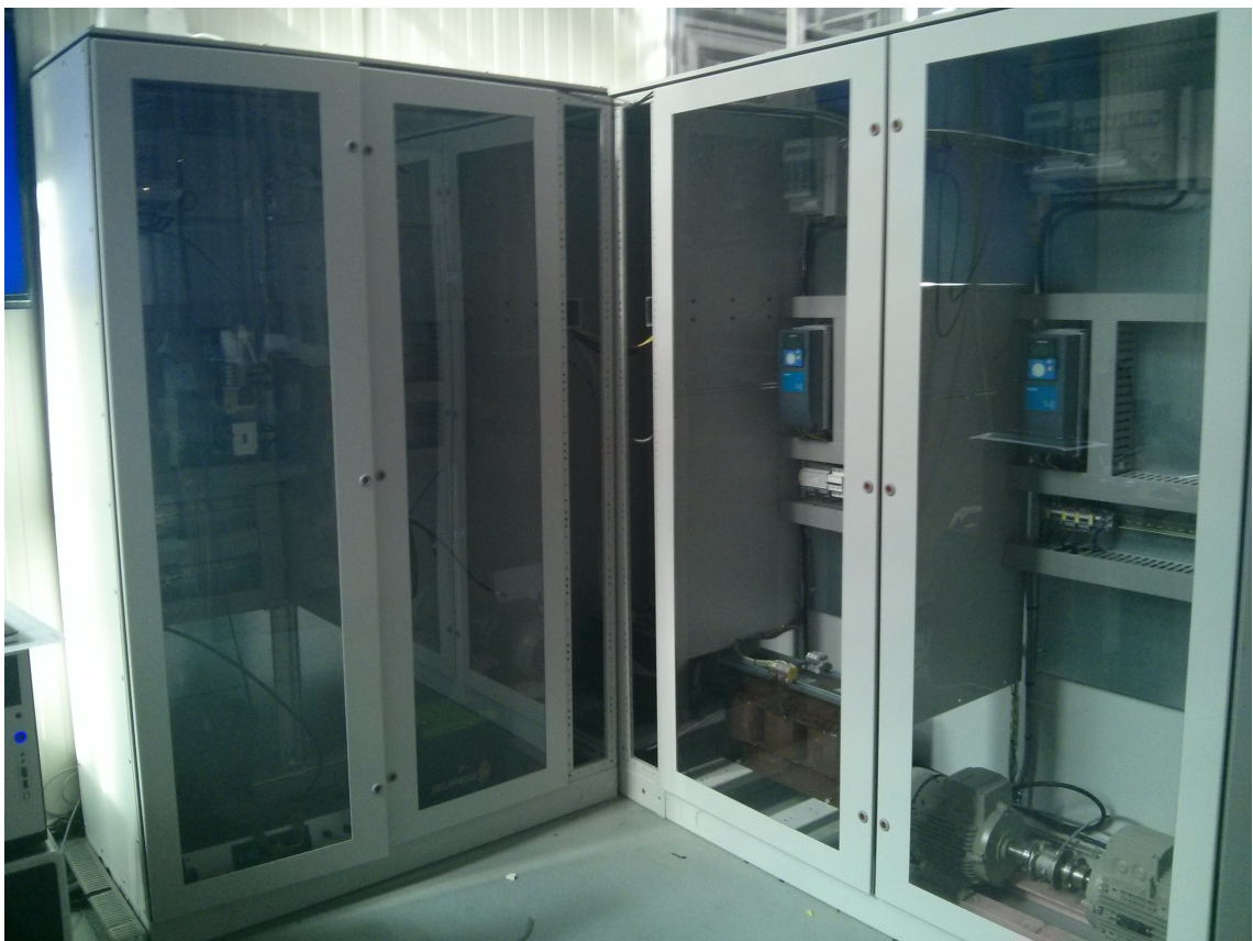
(b) Right hand side cabinet, showing PTO/PTI motor generator pair and battery location (not installed yet).
