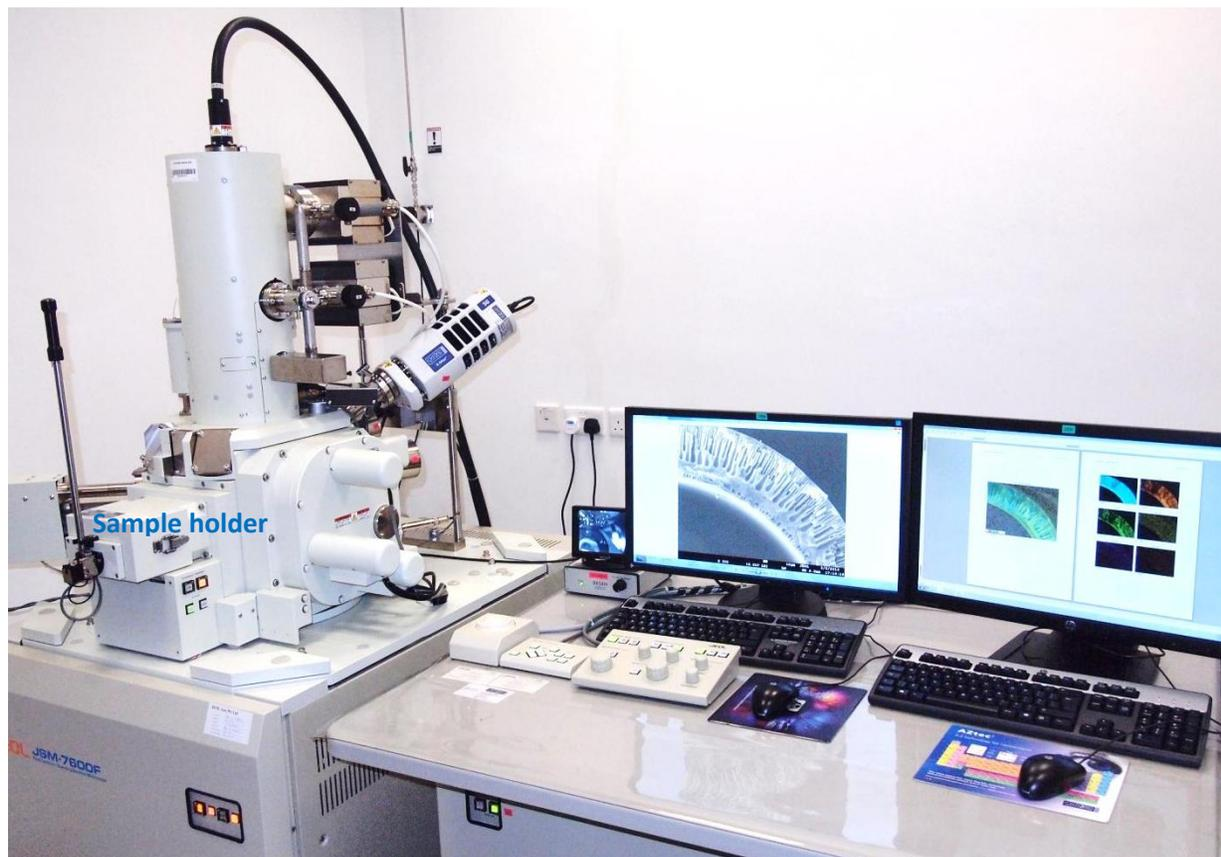
Figure.4.6. Scanning electron microscope (SEM) (Jeol Jsm-7600F) coupled to an XmaxN detector for energy-dispersive X-ray (EDX) analysis used in this study
