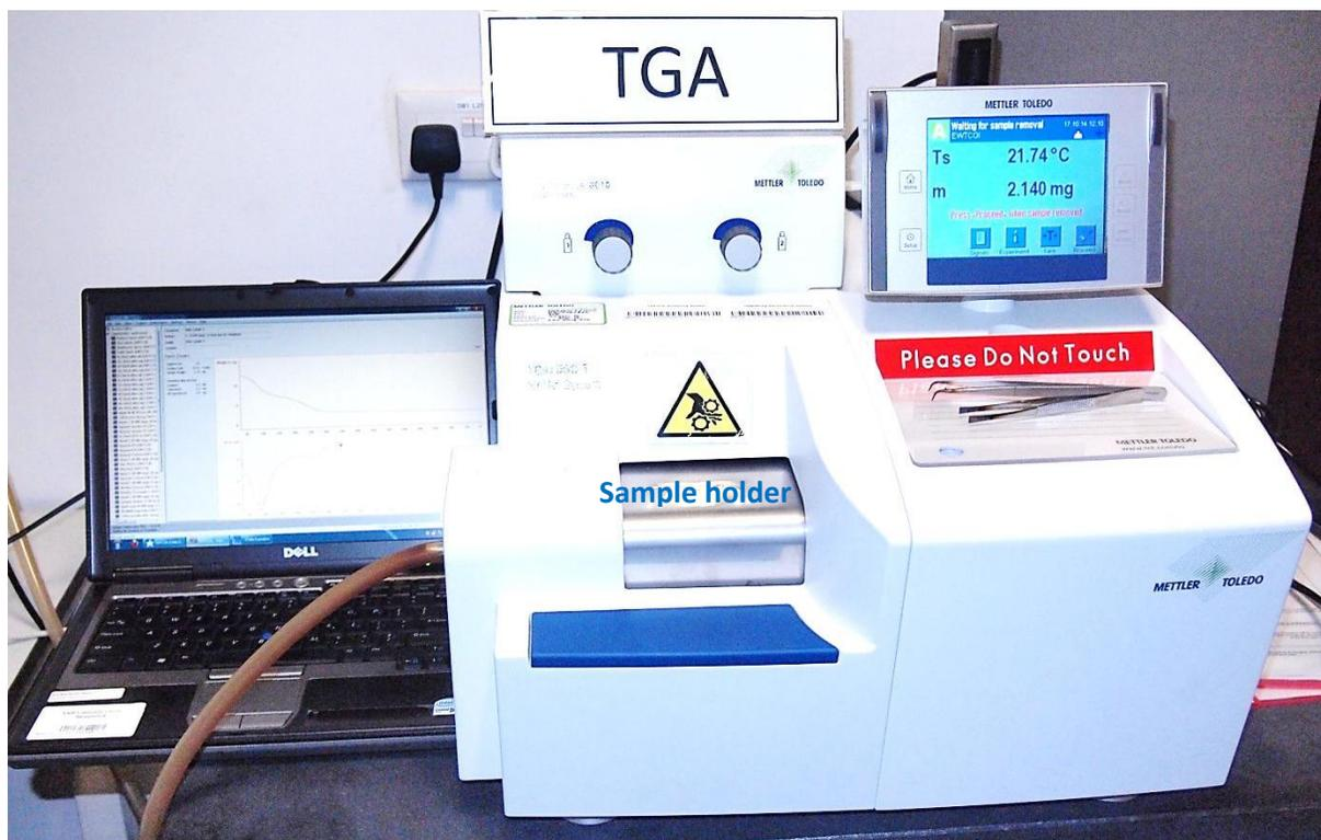
Figure.4.3. Thermo Gravimetric Analyzer (TGA5000, TA instrument) used in this study
