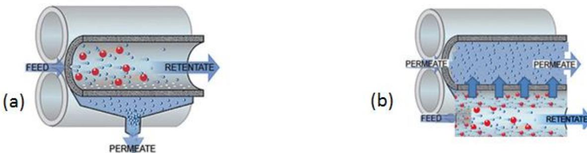
Figure.2.4. (a) Inside-out filtration, (b) outside-in filtration
