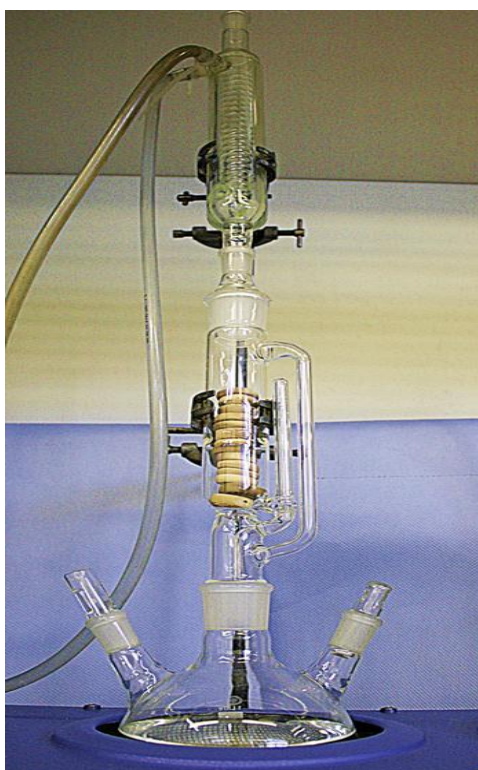
Figure 3.4: Diagram of Soxhlet system for washing polyHIPE
