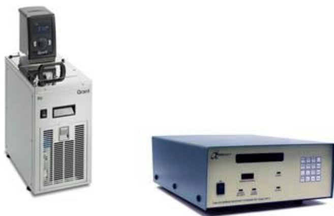
Figure 4.2 – Grant Optima T100 R water saturation system and Alpha Moisture chilled mirror hygrometer
