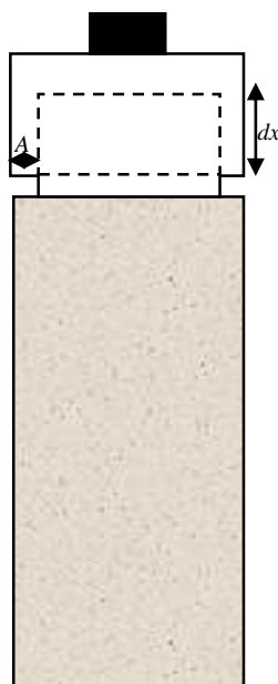
Figure 3.2. An illustration of empty batch vial showing the gap length ( dx ) and the cross-sectional area ( A ) of the assumed gap between the Mininert cap and the wall of the vial.
