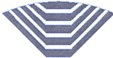
Fig. 2.5 Cross Section of one Segment of an Axially Laminated SRM
