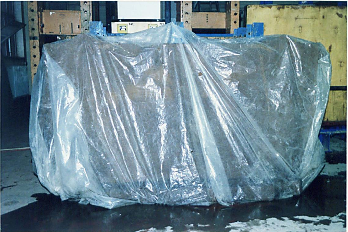
Fig.6.10: A beam being cured with the control specimens
