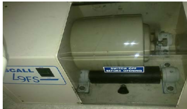
Figure 4.1 Ball mill machine that was used in the milling process of AW powders.
