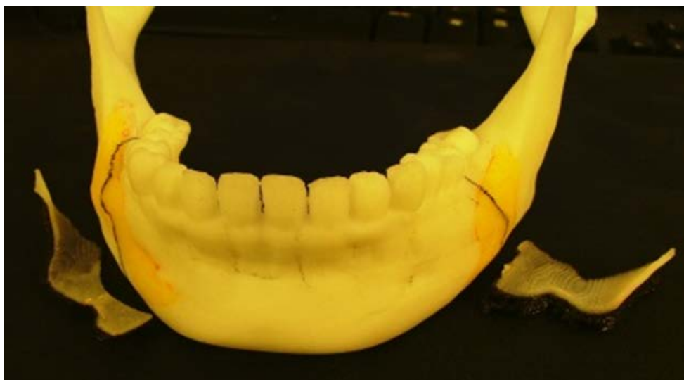
Figure 5.16 FDM model of the fixation plate for form fitting test.
