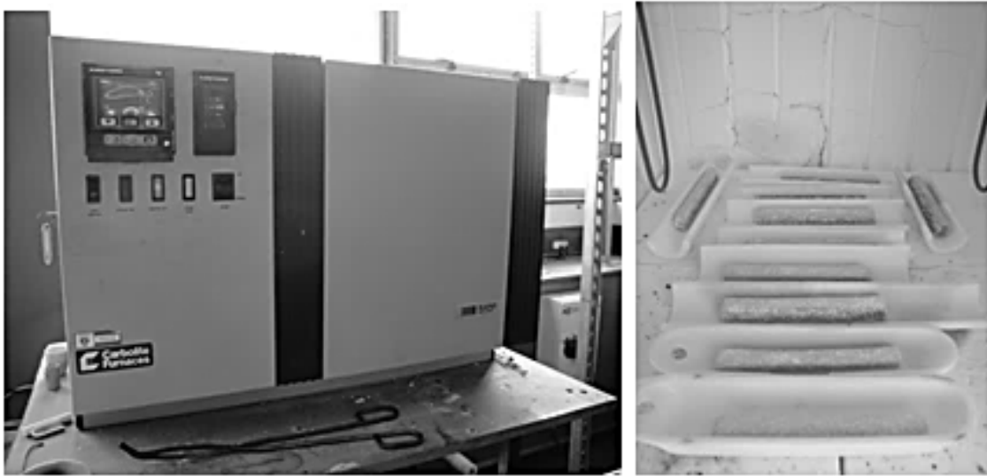
Figure 4.10 Equipment used in sintering AW green parts.
