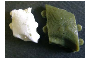
7. Comparing the fabricated AWGC artefact with the wax pattern.
