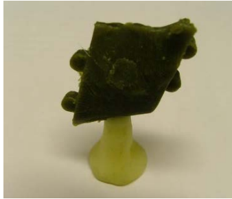
1. Preparing the wax pattern for LWC. Attaching the spru.
