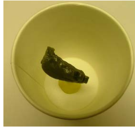
2. Setting the assembly inside a container. Cerrostone plaster is then poured in and let to set overnight.
