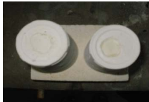
4. Wax pattern was removed by inverting the cast and heated in oven before AWGC-PMMA powder was filled into the cast.
