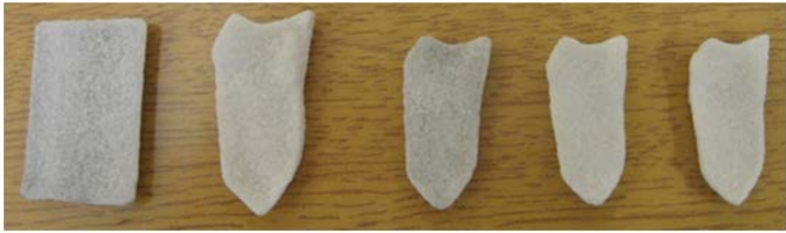
Specimen A Specimen B Specimen C Rectangular Slab 20% Enlarged Patch Patches as the same size as original CAD model
