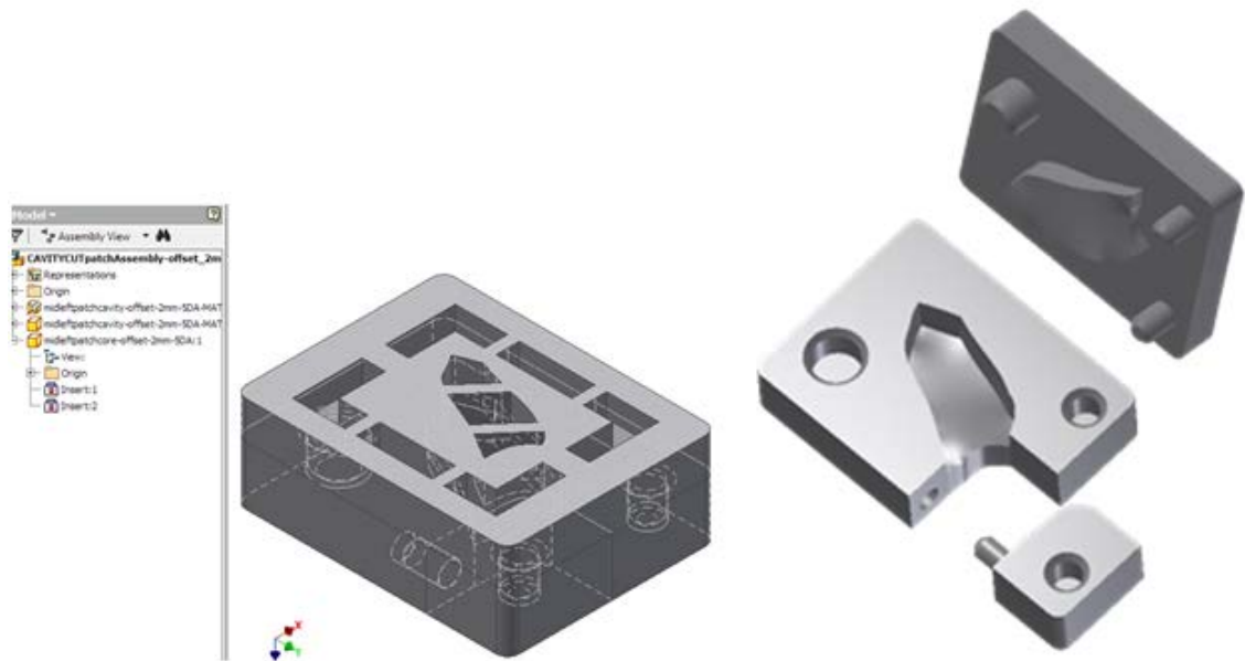
Figure 5.18 CAD model of the moulding assembly and exploded view.
