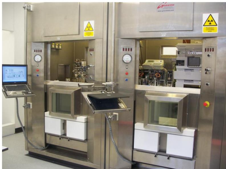
**Figure 12: Hot-cells (Gravatom) within the Sir Bobby Robson Foundation PET Tracer Production Unit at Newcastle University.**
