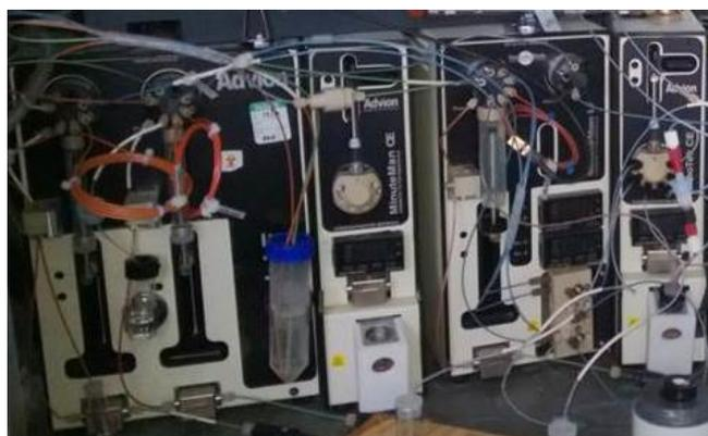
**Figure 13: A commercially available microfluidic synthesis system (NanoTek<sup>®</sup>, Advion Biosciences, Inc., Ithaca, NY).**
