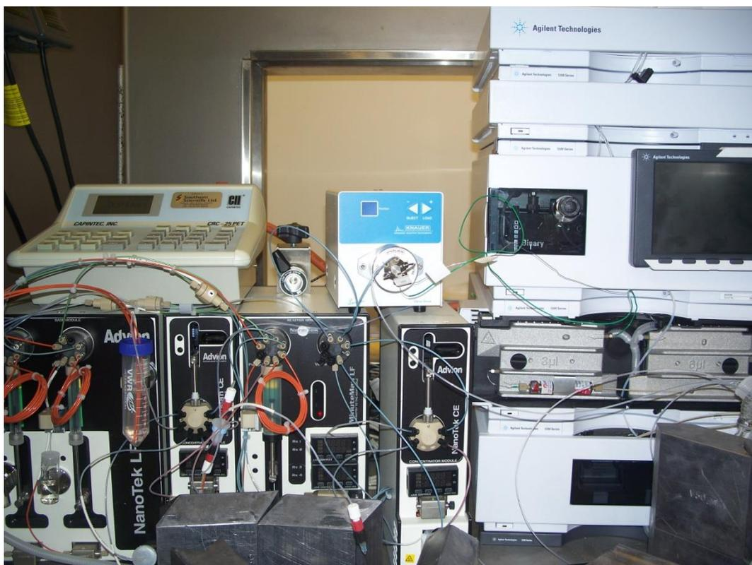
**Figure 45: Advion NanoTek (BM bottom left, RM middle and CM right), auto-injection valve (blue box) and Agilent Technologies 1200 series in-line HPLC.**
