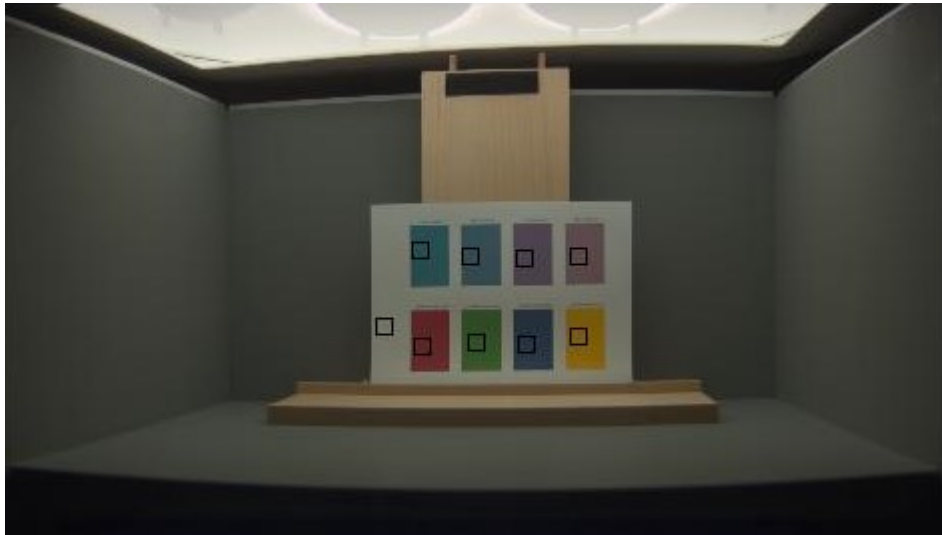
Figure 2.13. Rasterisation of a hyperspectral image, of a printed test sheet under uniform illumination; black squares mark the area over which spectra were averaged.
