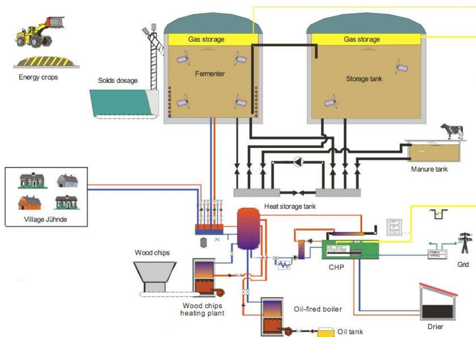
Figure 4. Diagram of Jühnde Bioenergy system (IEA, 2009b)
