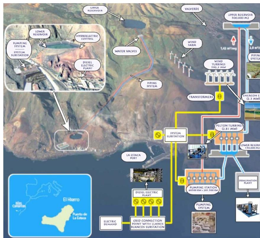
Figure 5. El Hierro Wind-Hydro system. Source: Hallam et al (2012, p.2965)
