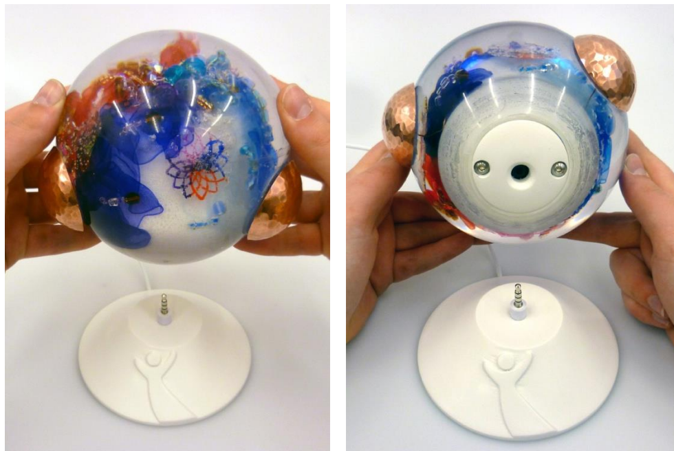
Figure 27. Bottom of the Sphere showing the small button head cap screws and the indentation in the middle for the charging plug.
