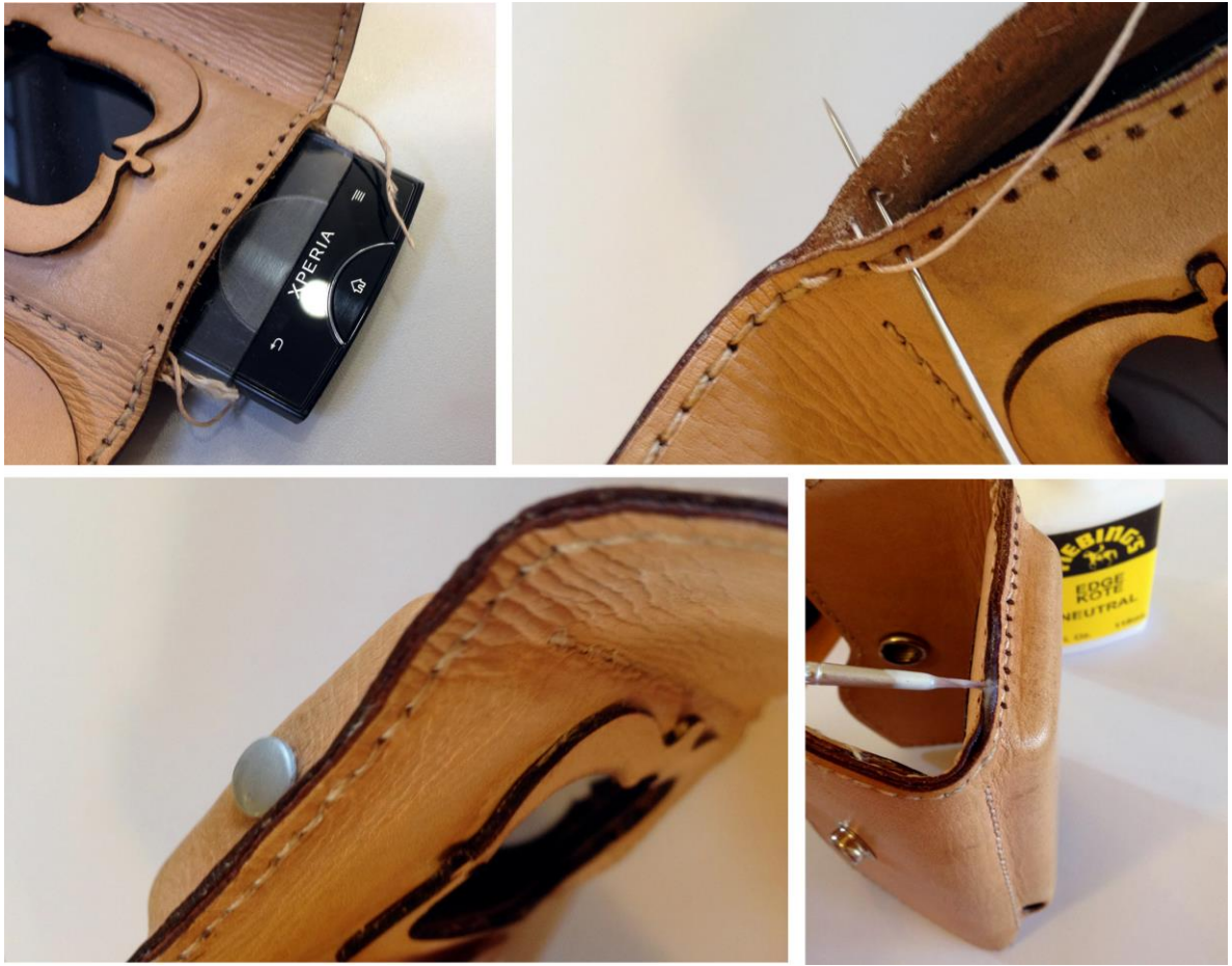
Figure 31. Shows the transparent Perspex Sheet that protects the phone screen, with the device being moulded into the leather cover, and its individual layers being stitched and glued together tightly.
