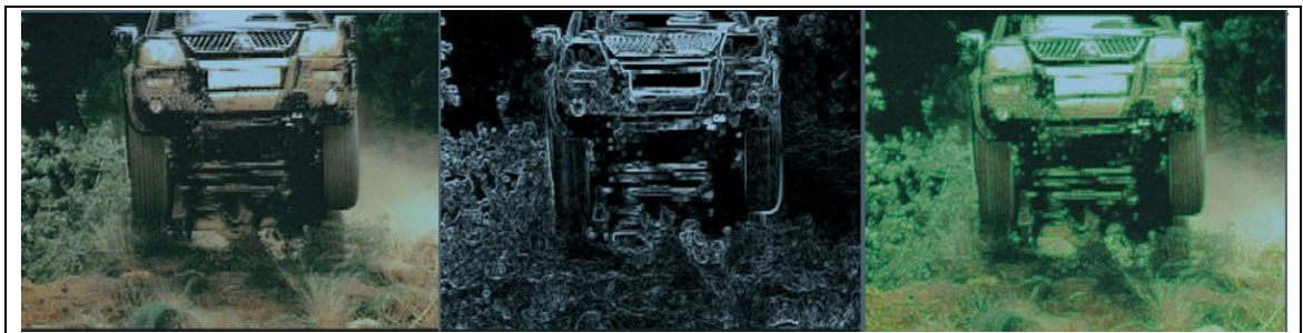
Figure 1-17 Television image enhancements. Left: Original image, Middle: the detected edges and Right: the edges coloured and overlaid on the original television image [93]
