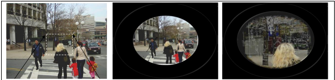
Figure 1-19 The output of Peli's vision enhancement system (RP). Left: Original scene. Middle: Demagnification assists in seeing the whole field of vision, but losing the high resolution central vision. Right: Superimposed edge images enhance visibility in the central area, while the full field of view is maintained [94]
