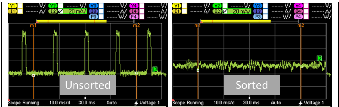
Figure 4-16 The current drawn by the optoelectronic micro-LEDs, by continuously sending a frame containing all pixels with an intensity value equal to 1. (Left) data sent using direct PWM (Right) data sent using an even power distributor
