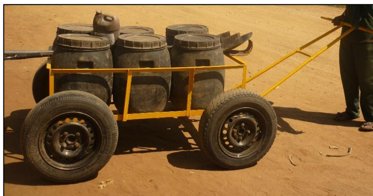
Figure 4-9: Manual faecal sludge removal and transportation equipment in use in Kanyama 4
