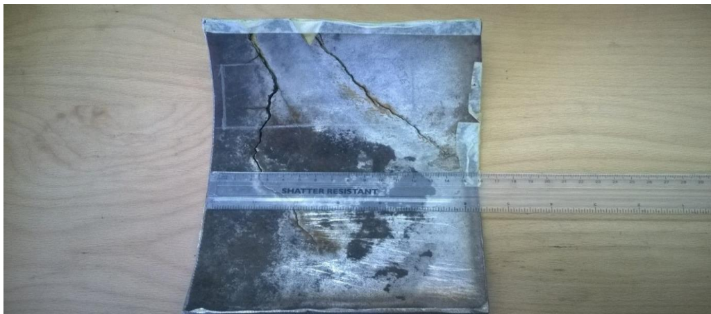
Figure 6.15: Photograph of Steel Sample with Stress Corrosion Crack
