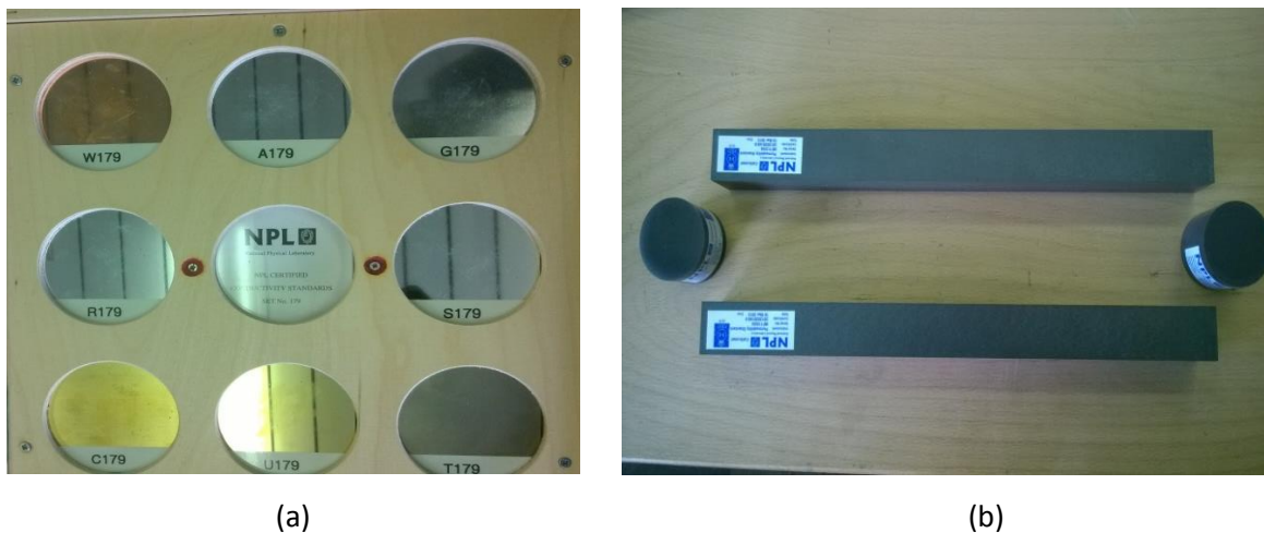
Figure 4.11: Experimental Validation Samples. (a) Photograph of Conductivity Samples. (b) Permeability Samples
