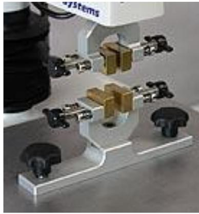
**Figure 3 “Miniature tensile grips”. Photograph. n.d. Texture Technologies Website. Reproduced by kind permission by Texture Technologies Ltd.**
