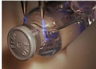
Figure 6.2 - Vial undergoing HVLD [159]
