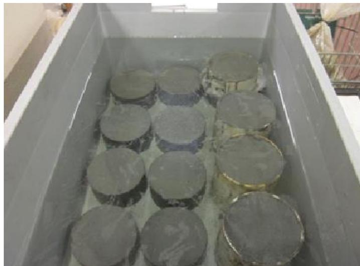
*Figure 4-5 : Water curing of grout specimens*
