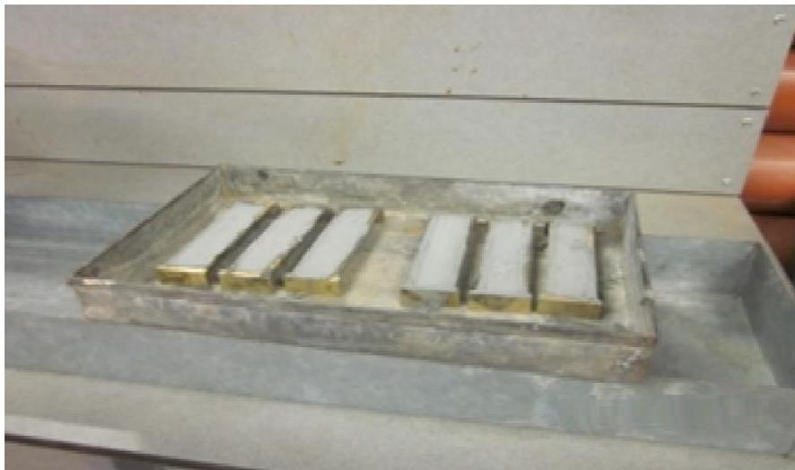
*Figure 4-7 : Shrinkage measurement using brass moulds*
