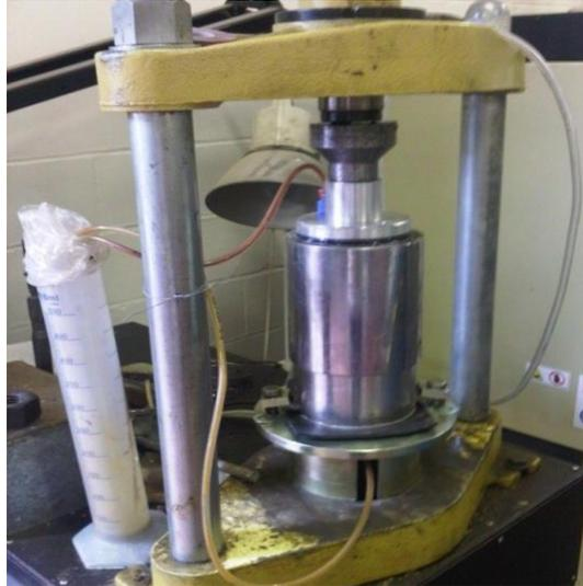
*Figure 3-7 : The consolidation cell*
