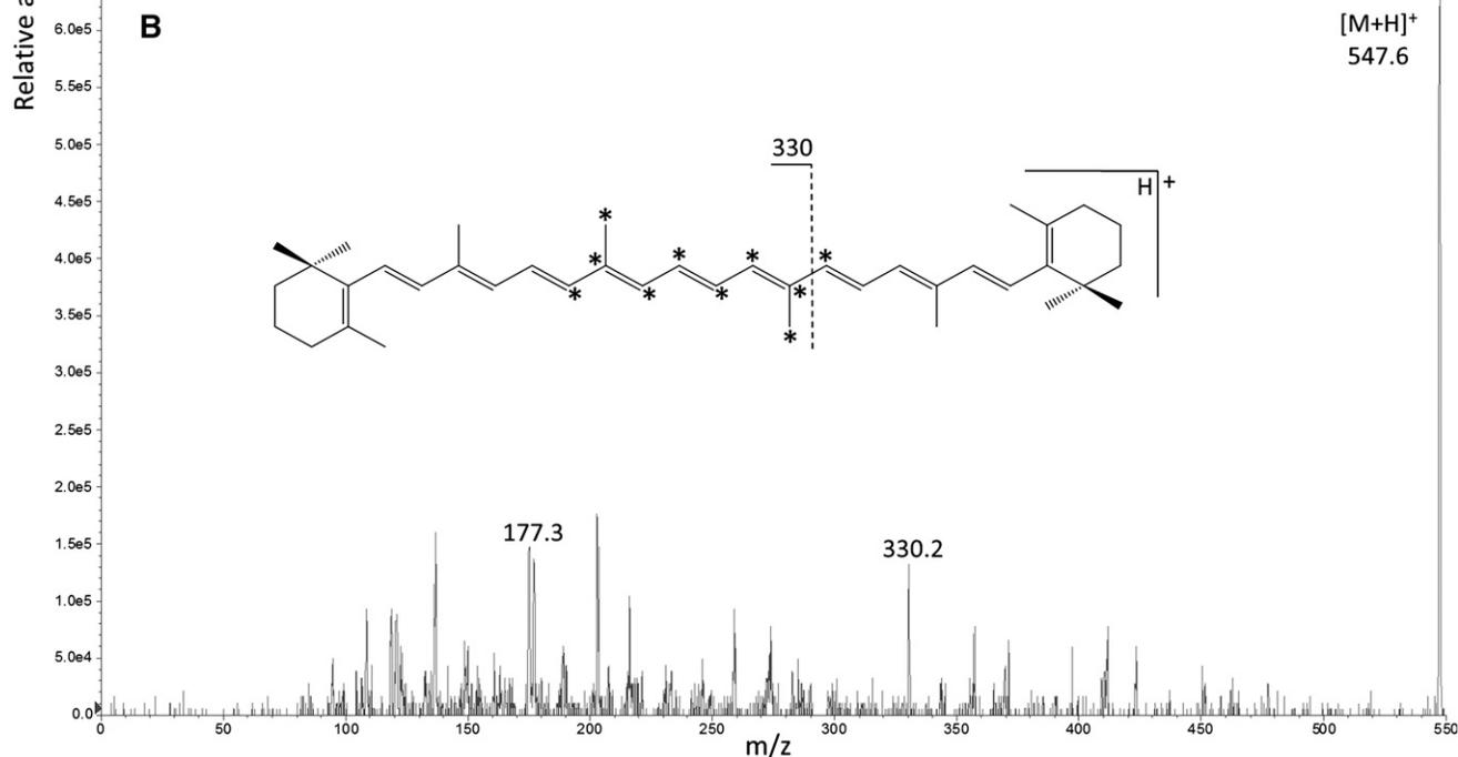
**Fig. 3.** Flow-injection APCI-MS/MS product ion mass spectra of  $m/z$  537 [ $^{12}\text{C}$ ]β-carotene (A) and  $m/z$  547 [ $^{13}\text{C}_{10}$ ]β-carotene (B) in positive mode. Asterisks (\*) denote position of [ $^{13}\text{C}$ ] labels.
