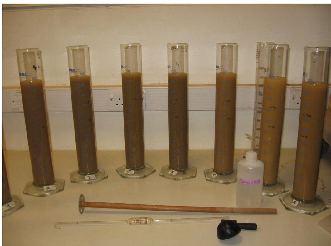
**Figure 6.2** *Measuring cylinders used during sedimentation of the soil samples*
