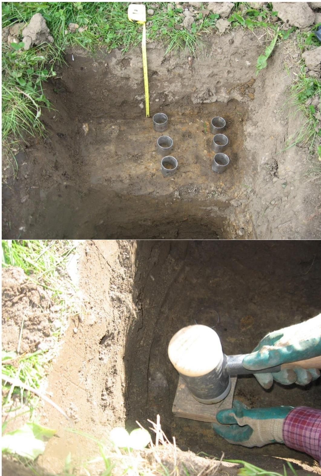
**Figure 6.1** *Collection of undisturbed soil cores using stainless steel rings in the soil profile.*
