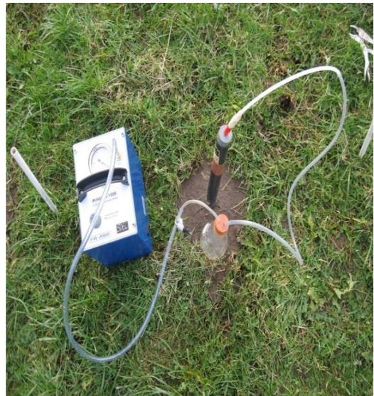
c) Plot layout with source area outlined by cup    d) Sampling of soil solution collected
