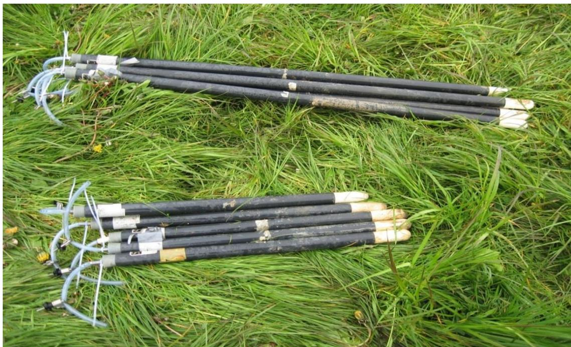
**Figure 7.4** Porous ceramic cups attached to sampling tubes as used in the experiments.
