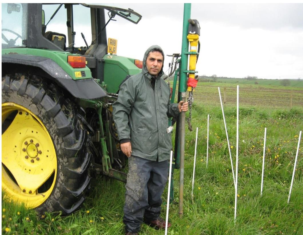
**Figure 4.1** *Hydraulic soil sampler in use in the field to collect soil cores*
