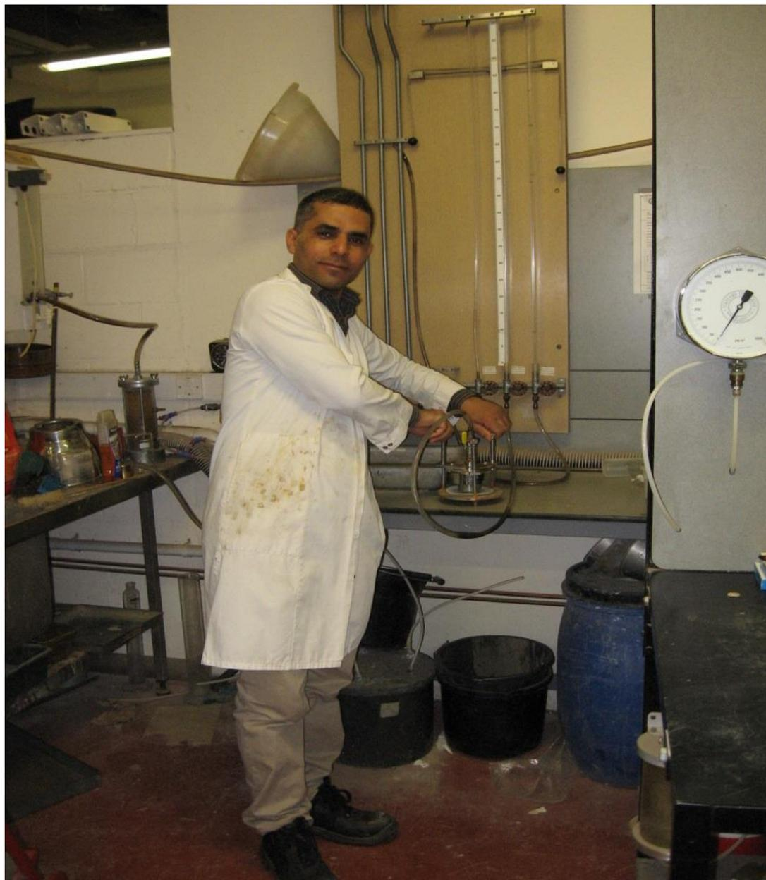
**Figure 6.3** *Measuring  $K_s$  of intact soil cores using the falling head method.*
