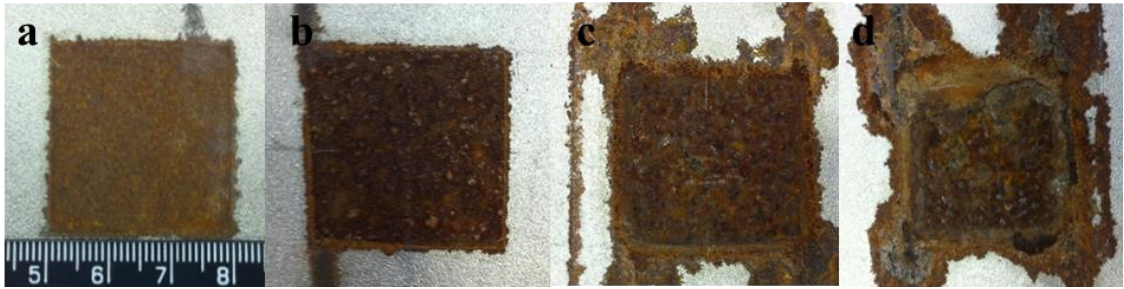
Figure 4.8 Images of corrosion samples after exposure periods of (a) 1 month; (b) 3 months; (c) 6 months; (d) 10 months.
