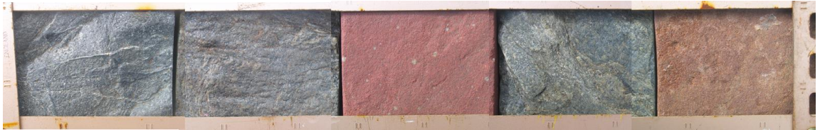
Figure 6-2: Frame 1 front showing igneous, metamorphic from Carradale, red sandstone, Loch Fyne metamorphic and yellow sandstone.
