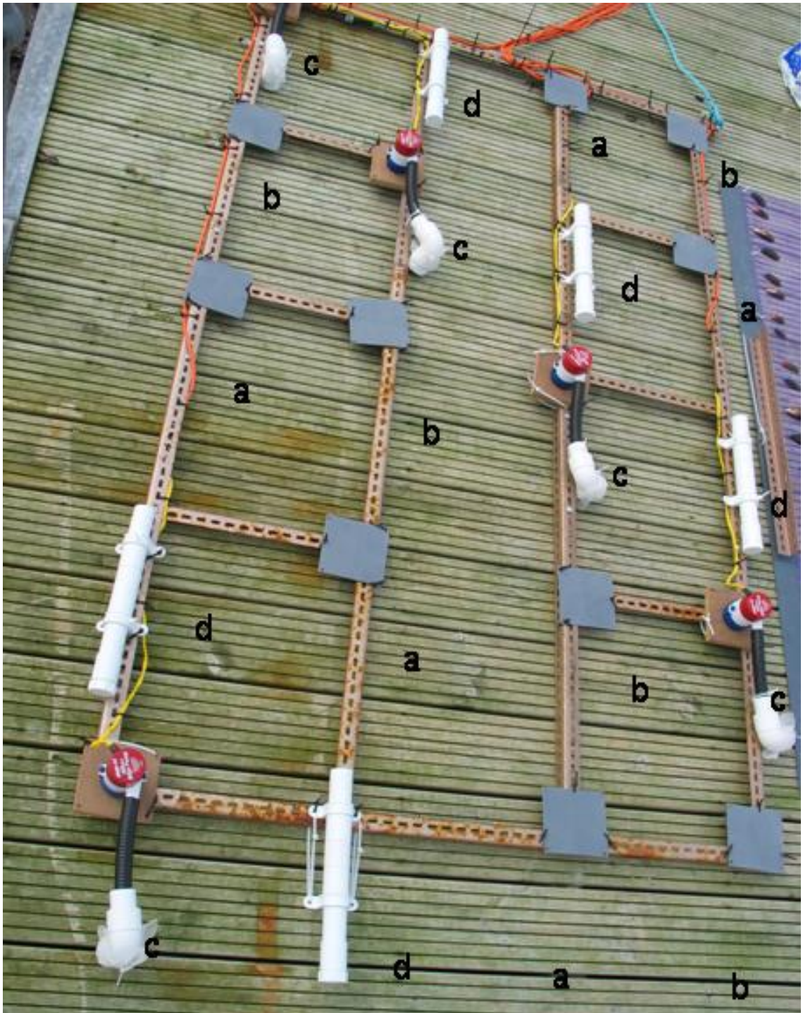
Figure 4-2 Photograph of Cyprid supply and settlement frame (a = plain settlement panel, b = adhesive settlement panel, c = pump, d = trap) in Latin square design.
