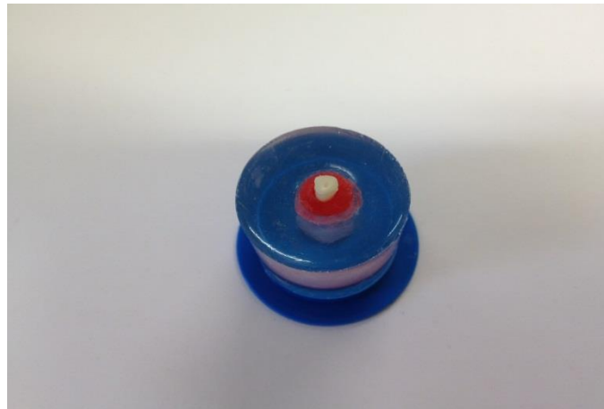
Figure 5.1. Cylindrical mould with a tooth mounted in soft red wax to hold it in position and create an apically closed system for irrigation.
