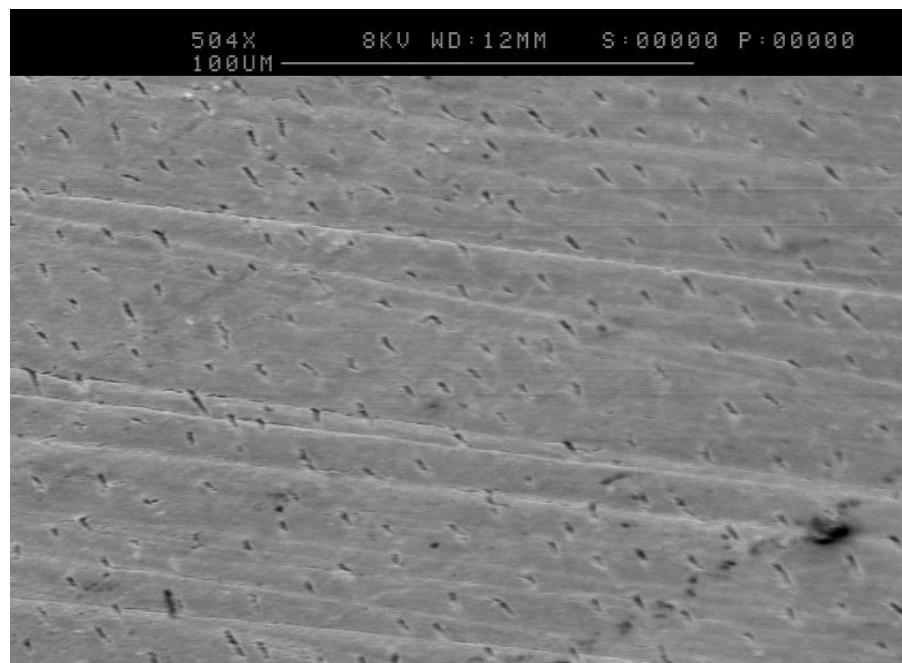
Figure 4.15. SEM image (500x magnification) to show representative Group 3 specimen after polishing with sand papers (1200 \mu m), and then with aluminium oxide (Hülsmann score 1).
