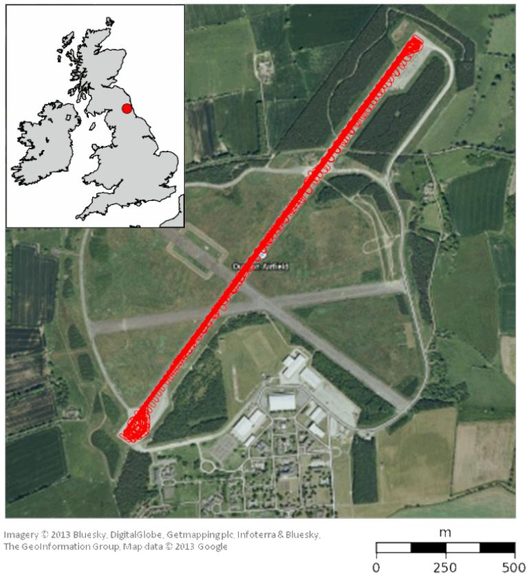
Figure 5.2: Location of the ‘kinematic’ dataset at Albemarle Barracks in Northumberland, United Kingdom. The trajectory of the vehicle on which the GNSS antenna was mounted is shown in red.
