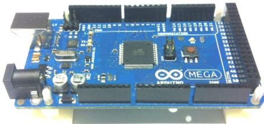
Figure 10.8 Microcontroller board type ARDUINO MEGA 2560
