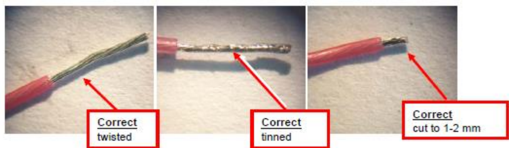
Figure 10.3 Wire stripped, twisted, tinned and trimmed [109]
