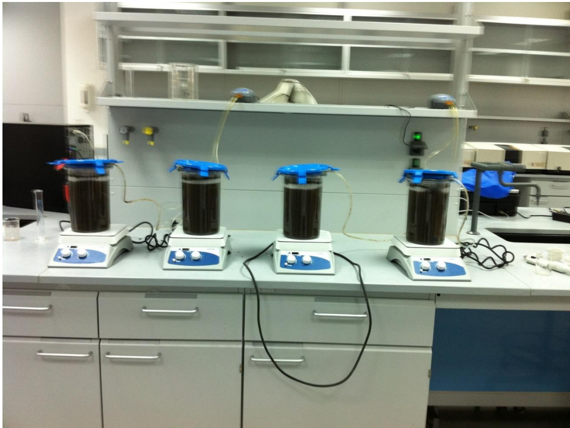
Figure 4.2: Photograph of the continuously stirred tank reactors.
