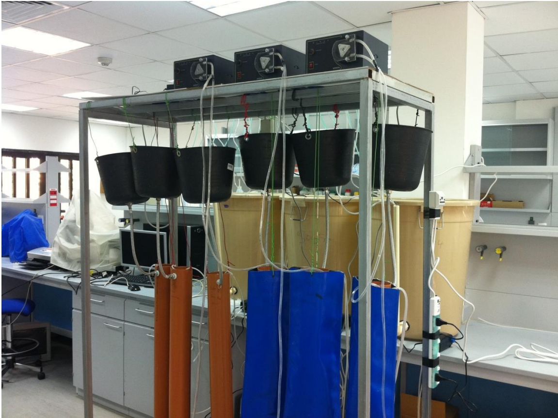
Figure 4.4: Photograph of the MBR (right) and SBR (left) reactors showing floor-standing reactors, suspended tanks and peristaltic pumps.
