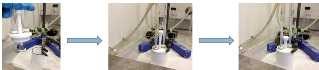
Figure 3.19. Etching steps of flat silicon surface by ammonium fluoride solution.
