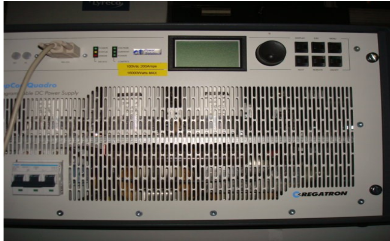
Fig. 3.7, TopCon DC power supply
