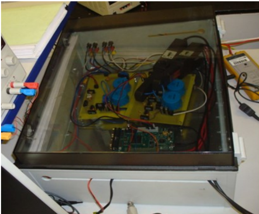
Fig. 3.12, DC-DC boost converter unit of instructed stand-alone PV system
