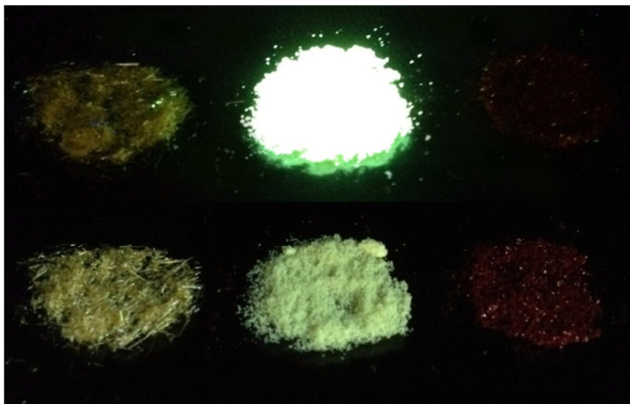
Figure 30 A picture of compounds 2 (left), 4a (middle) and 7a (right) under UV illumination (top) and in daylight (bottom). Clear luminescence is visible from 4a while all other compounds exhibit no such phenomenon.
