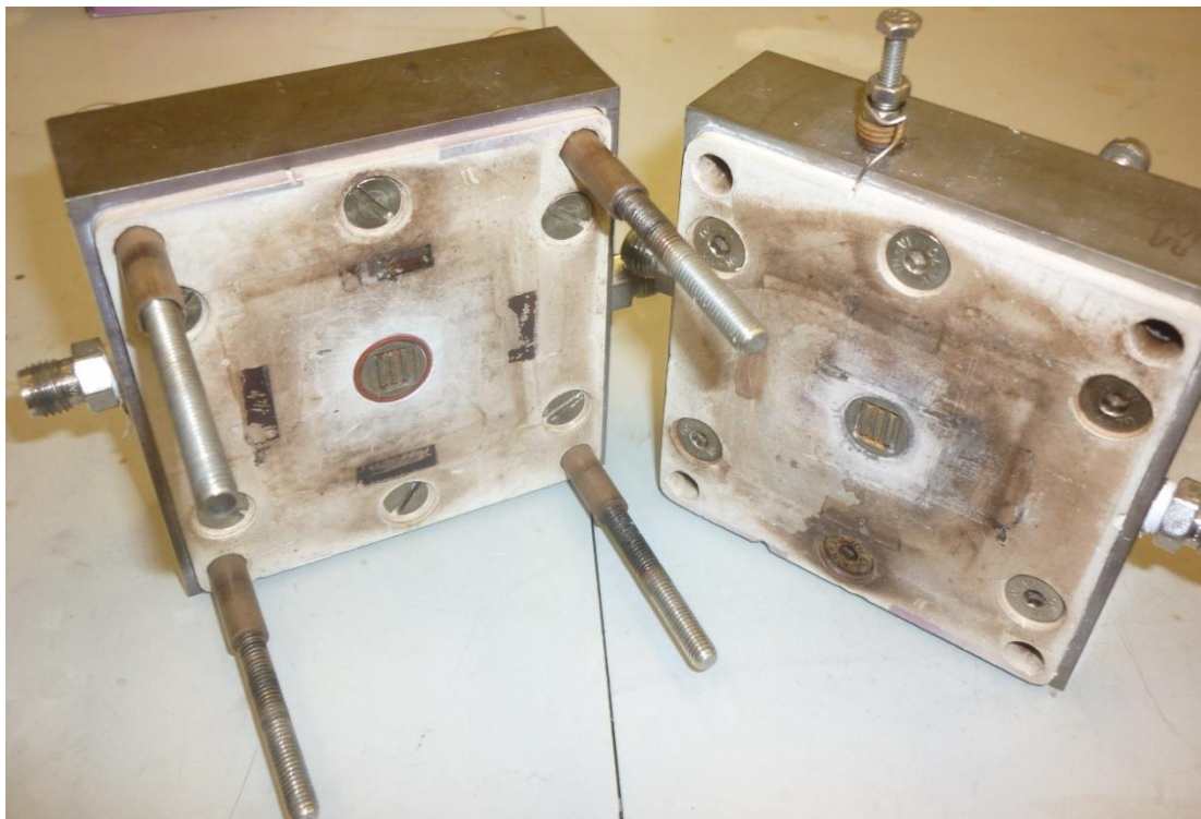
Figure 2-13 Photograph of the two halves of the unassembled polymer electrolyser cell
