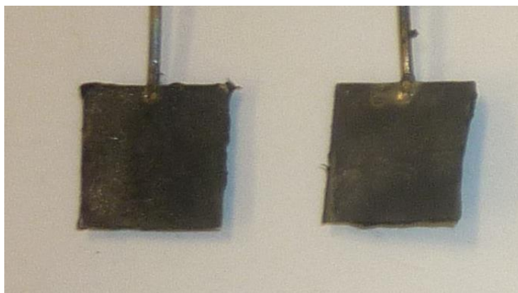
Figure 2-12 Two electrodes prepared with 25% PVDF after 30 minutes of oxygen evolution; Potential held at 1 V vs. Hg/HgO in 1 M NaOH at room temperature
