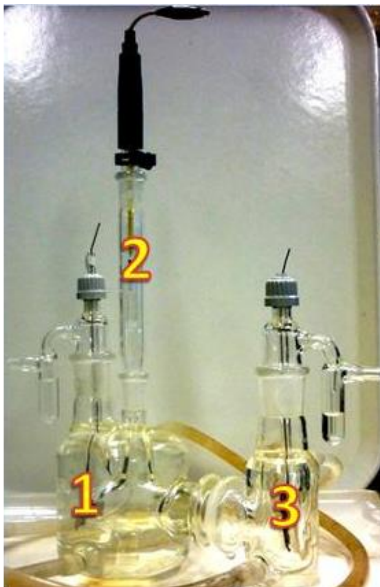
Figure 2-5 Glass half cell electrolyser with three electrodes; 1 working electrode, 2 reference electrode, 3 counter electrode
