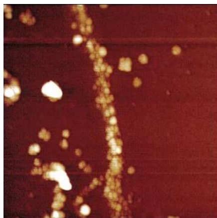
Figure 1-19: AFM image of a silver nanowire with granular structure.[18]
