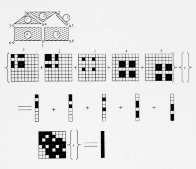
Figure 3.6: Structural finite element assembly calculations
