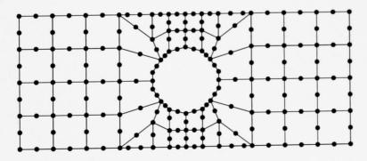
Figure 3.7: 2D finite element mesh
