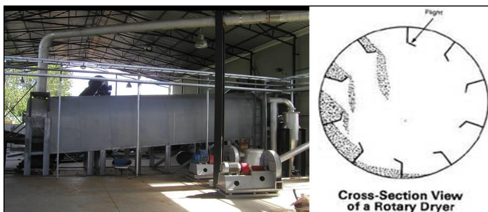
Figure (2.6): Picture and cross section schematic of the dryer (Calkan, 2007).
