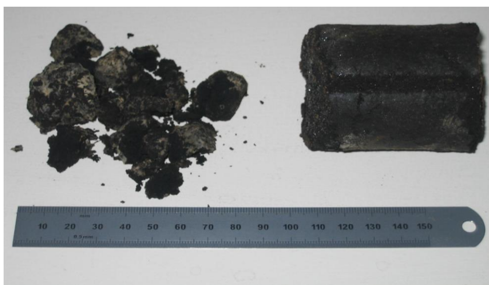
Figure (4.1): Initial and briquetted appearance of 70 wt% oil sludge and 30 wt% sawdust
