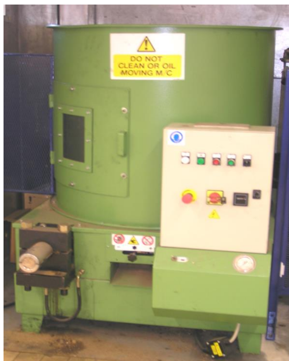
Figure (3.5): 100 kg/h capacity briquetter supplied by Por Ecomec SRL.
