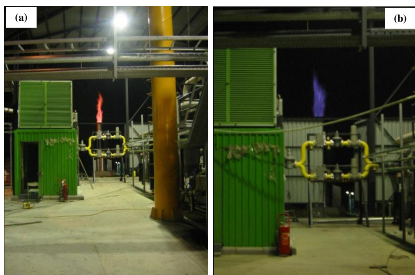
Figure (4.42): Visual demonstration of the tar cleaning effectiveness by the method carried out with 1 MWe scaled-up gasifier. Colour of the flare (a) before syngas cleaning, (b) after syngas cleaning
