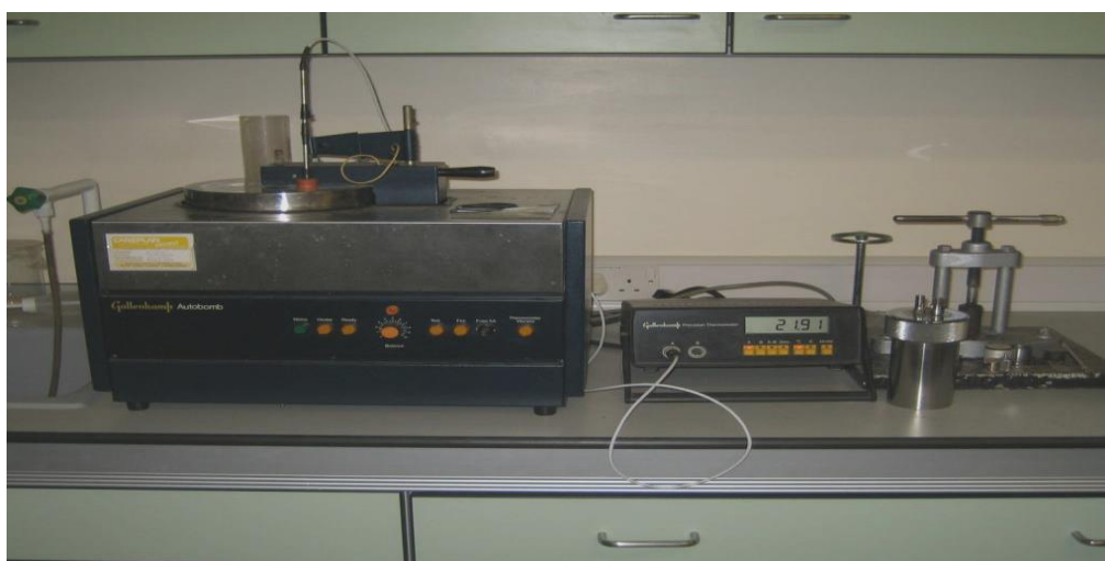
Figure (3.23): Actual bomb calorimeter set up used to perform the analysis
