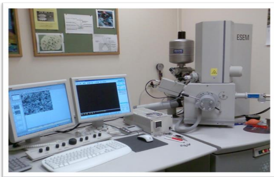
Figure (3.30): Scanning Electron Microscopy-Energy Dispersive X-ray (SEM-EDX) Analysis (Electron Microscopy Services at the Advanced Chemical and Materials Analysis (ACMA) Centre in Herschel building, Newcastle University).
