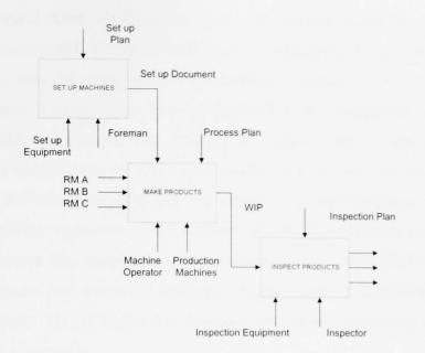
Figure 3.7: Basic Construction of an IDEF model
